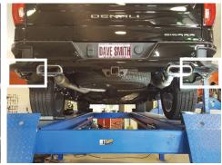
4. Unplug passenger and driver side sensor wiring then remove brackets from vehicle. Retain them for later use.
