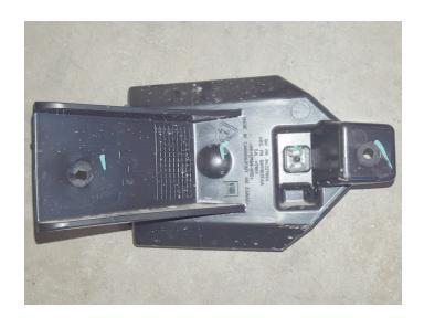
5. Remove screws (x3) securing passenger side bezel. Complete this step for driver side as well.
