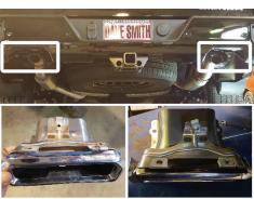
6. Remove nuts (x2) from driver side tailpipe flange. Then remove isolator and bolt from frame and disassemble tailpipe from vehicle. Retain isolator and bolt for later use.
