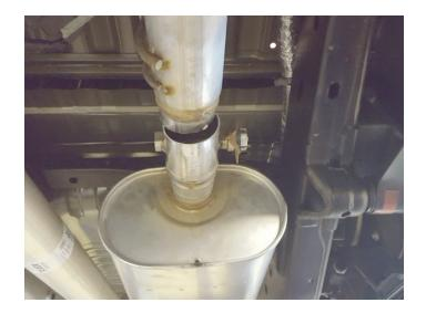
8. Disassemble tailpipe wire hangers from rear isolators then remove remaining tailpipe from vehicle. Retain isolater and bolt for later use.
