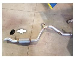
9. Disassemble inlet pipe wire hanger from isolater. Loosen factory clamp at catalytic converter and remove remaining muffler assembly from vehicle.
