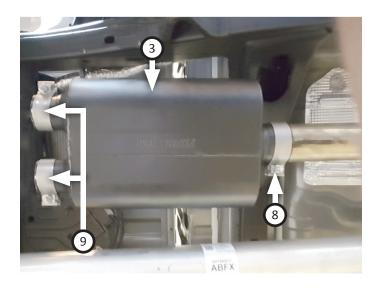
15. Route **right front tailpipe (4)** and **left front tailpipe (5)** over axle and connect them to muffler outlets. Mount wire hangers into isolators then tighten clamps enough to allow for adjustment.
