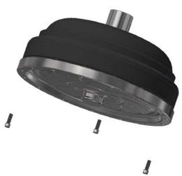
19. With three bolts installed and the pump drawn down all the way, you can now flip the converter over to access the remaining 12 bolts. Install all the 1/4-28 X 3/4" bolts and torque them to 10 ft-lbs. This completes the converter assembly process.
