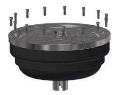
3. Next, insert the three extraction pins (included with kit) into the tapped converter bolt holes.
