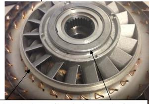
Stator placed on top of larger bearing and smaller diameter thick bearing placed on top of stator (this side up)
