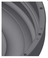
17. With the front, piston and table sitting on the table as depicted, align the marks on the pump and the front while carefully lowering pump onto front and resting it on the o-ring.
