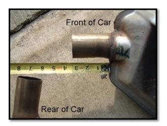
Step #2: Remove stock mufflers and remove burr or rough metal from edge of the stock exhaust tube.
