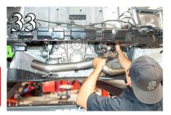
WARNING: Use extreme caution during installation. Torque all fasteners according to manufacturer's torque values and tightening sequence. <u>DO NOT</u> use impact tools to tighten fasteners on Borla Performance Exhaust Systems. Use of such tools may result in bent flanges or gasket contact areas leading to exhaust leaks.
