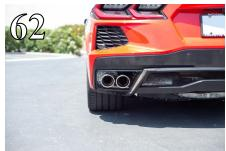
NOTE: When you first start your vehicle after the installation of your new Borla Performance Exhaust System, there may be some smoke and fumes coming from the system. This is a protective oil based coating used in the manufacturing of mandrel bent performance exhaust tubing. This is not a problem and will disappear within a very short period of time after the exhaust has reached normal operating temperatures.
