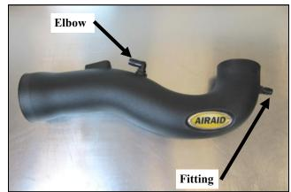
**6.** Install the Barbed Fitting and Elbow into the Airaid Intake Tube. Apply the Airaid Decal onto the Tube as shown.
