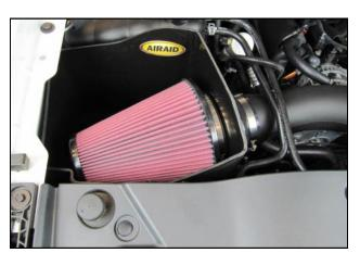
**13.** Install the Airaid Premium filter onto the Filter Adapter, and tighten the hose clamp.
