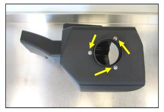
**4.** Install the Filter Adapter onto the Cold Air Box as shown using the three 1/4-20 Button Head Screws and 1/4" Flat Washers.
