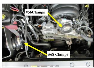
**8.** Slide the Hump Hose with the #68 Hose Clamps onto the Filter adapter and the coupler and the #56 Clamps onto the throttle body. Leave the clamps loose
