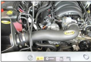
**9.** Install the Airaid Intake Tube into the Hump Hose and couplers. Adjust for fit and tighten all four Hose Clamps.
