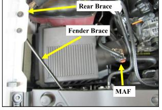
2. Using an open end wrench, remove the passenger side fender brace and set it aside. For ease of installation, remove the rear brace bolt and set it aside. Unplug the Mass Air Flow sensor, or MAF and un anchor it from the airbox. Unseat the airbox from it's mounting grommets and remove the factory airbox.
