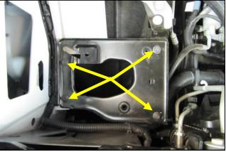
**3.** Remove the 4 bolts in the airbox mounting tray and set them aside. They will be reused in step **5**. Remove the Tray, it will not be re used.
