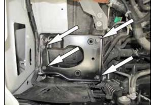
5. Install the AIRAID® air box into the vehicle and secure with three of the OEM bolts from step #3. Apply one of the provided AIRAID® decals to the air box as shown.
