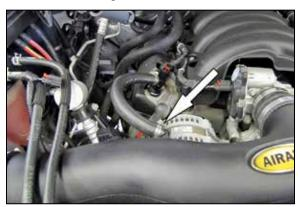
11. Install the provided PCV hose onto the fitting on the valve cover and in the intake tube with the provided hose clamps. Secure the PCV hose with the hose clamps.
