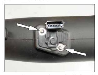
7. Remove the OEM mass air sensor from the factory air filter housing and install it into the AIRAID® intake tube and secure with the provided hardware.
