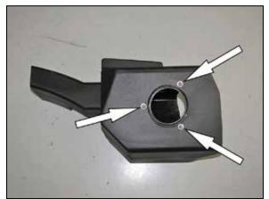
6. Install the 3/8" NPT elbow fitting and 3/8" NPT plug into the AIRAID® intake tube where shown. Apply the provided AIRAID® decal onto the intake tube where shown.
