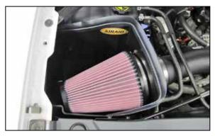
14. Install the weather strip onto the top edge of the AIRAID® air box with the contour rolling away from the filter as shown.
