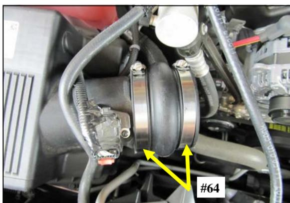
5. Slide the Hump Hose and #64 Clamps onto the factory air box. If you are installing an Airaid Jr. kit, install the Airaid Premium Filter at this time.
