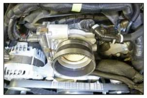
6. Install the provided coupler onto the throttle body. 5.3L engines will use the smaller coupler and 6.2L engines will use the larger coupler.
