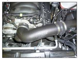
9. Install the AIRAID<sup>®</sup> intake tube into the hump coupler and then the coupler at the throttle body, adjust the tube for best fit and secure with the provided hose clamps.
