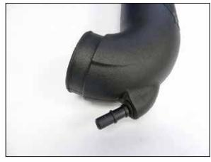
8. Install the provided grommet and quick connect fitting into the AIRAID<sup>®</sup> intake tube as shown.
