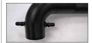
17. Install the two provided crank case vent fittings into the AIRAID intake tube as shown.
