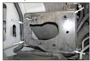
7. Remove the four bolts securing the air box mounting tray and then remove the tray from the vehicle.
