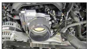
13. Install the coupling hose (08698 for 5.3L, 08497 for 6.2L) to the throttle body and secure with the provided hose clamp.
