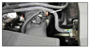
2. Disconnect the mass air sensor electrical connector.
