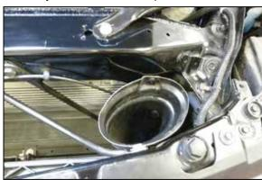
14. Push the factory fresh air intake duct into the AIRAID® air filter housing and then reinstall the plastic clip to secure it into position.
