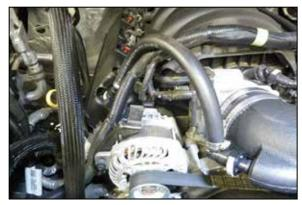
24. Install the AIRAID® air filter onto the filter adapter and secure with the provided hose clamp.
