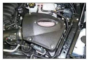
27. Install the AIRAID® air filter housing lid onto the air filter housing and secure with the provided hardware.
