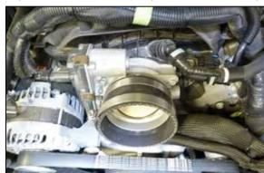
17. Install the coupler hose (KITRDCR05) onto the throttle body and secure with the provided hose clamp.
