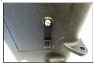
11. Install the provided wiring harness bracket onto the AIRAID® air filter housing and secure with the provided hardware.
