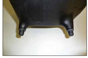
12. Remove the two factory mounting grommets from the factory air filter housing and install them onto the AIRAID® air filter housing.
