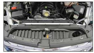
6. Release the ten plastic locking pins holding the upper radiator valence and then remove the valence from the vehicle.
