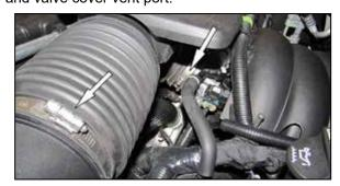
4. Loosen the hose clamps that secure the intake plenum assembly to the throttle body and air filter housing. Disconnect the plenum from the air filter housing and then rotate the plenum assembly counter clockwise to disengage the keyed mount and then remove the plenum from the throttle body.
