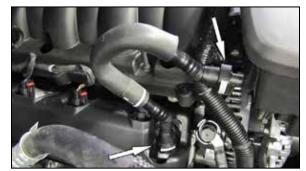
3. Depress the locking tabs and then disconnect the crank case vent line from the intake plenum and valve cover vent port.
