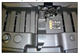
29. Reinstall the hood release arm to the hood latch and secure with the factory bolts.
