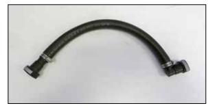
21. Assemble the crank case vent assembly using the provided hose, straight quick disconnect fittings and hose clamps as shown.
