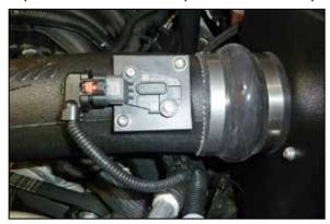
25. Reconnect the mass air sensor electrical connection. Use the provided tie wrap to secure the wiring harness to the A/C line with some slack for the wiring connector.
