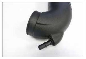
20. Install the grommet and quick disconnect vent fitting into the AIRAID® intake tube as shown.
