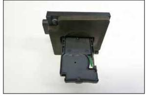
18. Install the provided gasket onto the provided mass air sensor adapter. Remove the mass air sensor from the factory air filter housing and then install it into the adapter and secure with the provide hardware.
