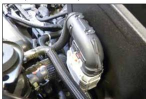
15. Clip the wiring harness onto the bracket installed onto the AIRAID® air filter housing.
