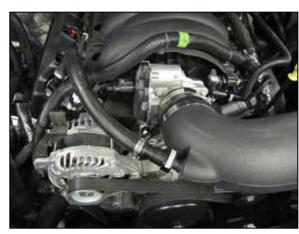
11. Connect the crankcase vent hose assembly to the fitting in the AIRAID® intake tube and to the valve cover port.
