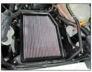
5. Remove the upper air filter housing and replace the factory air filter with the provided AIRAID® air filter and then reinstall the upper housing and secure with the factory hardware.
