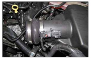
6. Install the provided hump coupler (KITHUMPHS22) onto the air filter and secure with the provided hose clamp.
