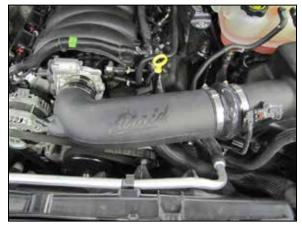
9. Install the AIRAID® intake tube into the coupler at the air filter housing and then into coupler on the throttle body, adjust the tube for best fit and then secure with the provided hose clamps.
