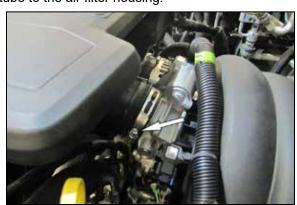
4. Loosen the hose clamp that secures the intake plenum to the throttle body. Rotate the plenum counter clockwise to unlatch it from the mounting bracket and then remove the plenum from the vehicle.
