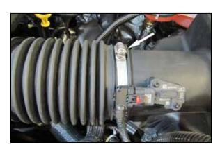
3. Loosen the hose clamp that secures the intake tube to the air filter housing.
