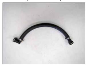
10. Assemble the crank case vent hose assembly as shown.
