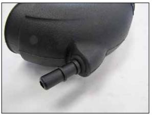
8. Install the provided grommet and vent fitting into the AIRAID® intake tube as shown.
