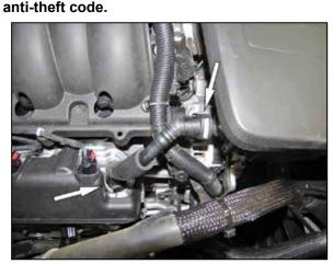
2. Depress the locking tabs and disconnect the crank case vent line from the intake plenum and valve cover.
