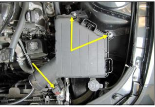
3. Disconnect the Mass Air Flow sensor. Using a deep 10mm socket, remove and save the two nuts that secure the factory airbox to the inner fender. These will be reused in step 10. Lift up and remove the entire airbox and scoop assembly.
