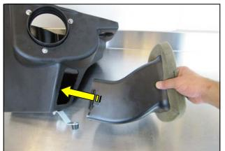
7. Transfer the factory air scoop into the Airaid Cool Air Box. When properly installed, the small locking tab will be inside the Box and the large one will be on the outside.
