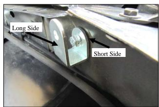
**9.** Install the Side Bracket (#12) where the ground lug was installed, using the 6mmx12mm Hex Bolt (#21), and Lock Washer (#19).
