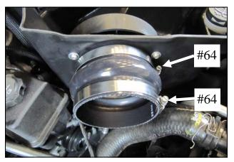
**13.** Slide the Hump Hose and two #64 hose clamps onto the Filter Adapter. Leave the Clamps loose at this time.
