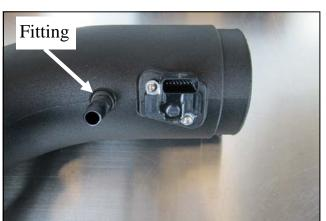
**14.** Install the 1/4" Barbed Fitting into the Airaid Intake Tube as shown. Transfer the Mass Air Flow meter from the factory air box, into the Airaid Tube and secure it using the two 8-32 x 1/2 Screws (#23). Do Not Use The Factory Hardware.
