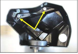
5. Transfer the two air box mounting grommets and steel sleeves from the factory air box into the Airaid Cool Air Box.
