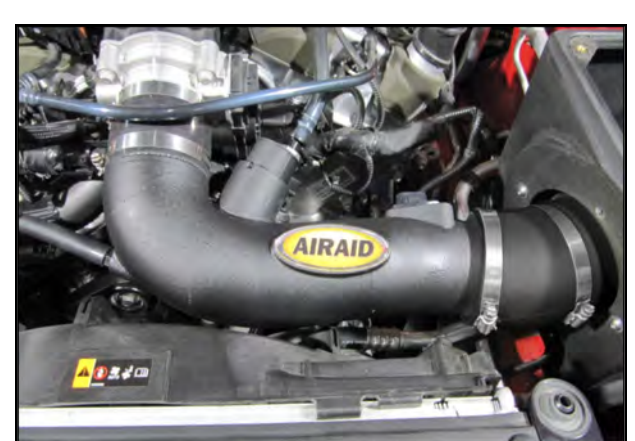
21. Insert the Intake Tube into the Elbow first, then into the Coupler. Tighten all four Clamps.
