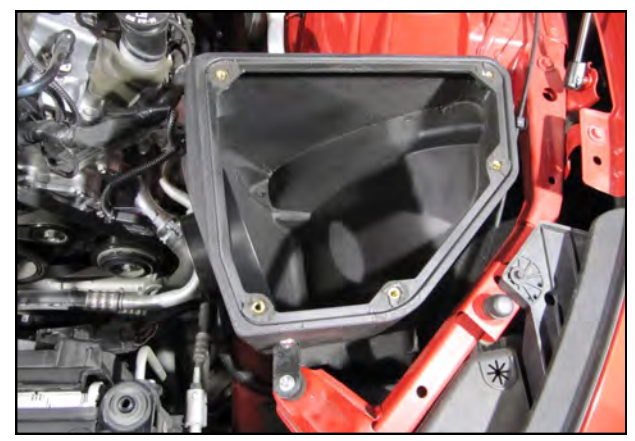
18. Place the Airaid Airbox assembly into the engine compartment as shown, with the mounting posts only fully seated in all three grommets.
