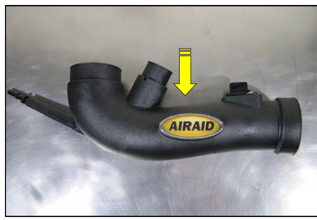
17. Prepare the Intake Tube for Badge installation by cleaning the mounting surface using a Prep Solvent or equivalent. Place the Airaid Badge onto the Intake tube as shown.
