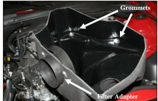
8. Reinstall the two steel sleeves and grommets into the Airaid Cold Air Box (CAB) (#4). Next install the filter adapter (#5) into the CAB as shown using three 1/4-20 button head bolts (#9), and 1/4" flat washers (#11). Refer to the line drawing above for details.
