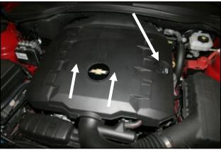
1. Disconnect negative battery cable. Remove the oil fill cap and then lift up on the front of the engine cover to remove it from the vehicle. Replace the oil cap for now to make sure nothing falls into the crankcase during the install.
