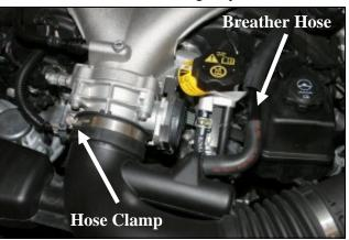
2. Disconnect the hard plastic crankcase breather tube from the rubber elbow. Leave the rubber elbow connected to the factory air intake tube. Next loosen the hose clamp that secures the air intake tube to the throttle body.
