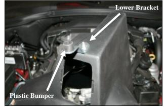
9. Turn the CAB upside down and mount the lower bracket (#24) to the bottom of the CAD using one 1/4-20x3/4" hex bolt (#10), 1/4" flat washer (#11), and 1/4" Nylock nut (#13) as shown. Next using one 8-32x5/8" button head screw (#17), and one #8 Kep nut (#18), attach the plastic bumper (#18) to the bracket as shown.
