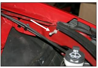
11. Using a 10mm wrench, remove and save the ground lug from the driver's side inner fender. It will be reused in step #13.
