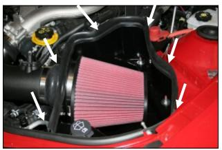
**18.** Install the Airaid Premium Filter (#1) onto the filter adapter and tighten the clamp. Next install the weather strip (#8) onto the top of the CAB. For ease of installation, start the front of the CAB near the radiator and work your way around towards the fender. Reinstall the engine cover and oil fill cap.
