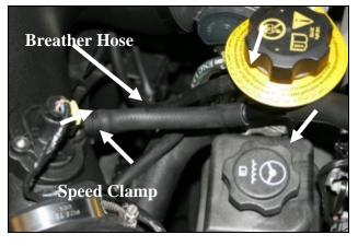
**17.** Install the 1/2"x 6" breather hose between the nipple on the air intake tube and the hard plastic crankcase breather tube. Refer to step #2. Install one #16 speed clamp (#20) over the breather hose at the nipple as shown.
