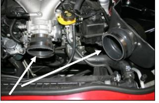
14. Install the hump hose (#7) onto the filter adapter using two #64 hose clamps (#22). Next install the reducing coupler (#5) with one #48 hose clamp (#21) on the throttlebody and one #64 hose clamp (#22) on the large end.
