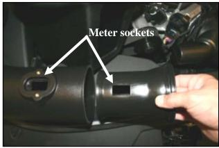
15. A) Insert the Modular Venturi Tube, (MVT), into the Airaid intake tube until it stops. Take care to align the MAF meter sockets, **B**) Reinstall the meter into the Intake-MVT assembly and secure using the two 8-32 button head screws (#16).
