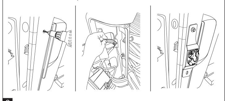
Allow the bracket to hang vertically. Using bracket as a template, mark (Center Punch) the upper hole of the lower slot (indicated). Pre drill hole with 1/8" drill bit, losen upper mounting hole and rotate bracket away from hole and open hole using a 21/64" drill bit. Remove burs, apply primer to edge of holes, and allow primer to dry. Install brackets.
