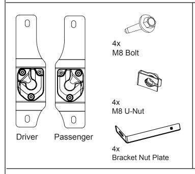
Assemble U-Nuts on to bracket plates in the orientation shown.
