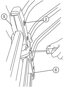
NOTE: Do not over tighten as this may strip out. Fastener will reach a noticable stopping point.
