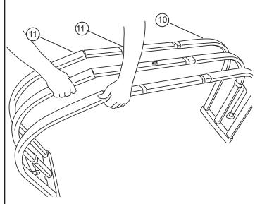
Adjust the width of the BEDXTENDER by placing the pivots into the mounting brackets. To keep overlap consant, adjust each tube so that the gap between the edge and the tape is the same.
