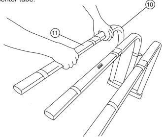
Connect the two halves. Make sure there is at least 3" overlap with the bent tubes on each side.
