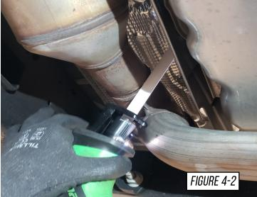
Then use a deburring tool on the cut end of the catalytic converters. It is important that the cut on the catalytic converters are smooth and there are no burs or sharp edges, as shown in **Figure 5.**
