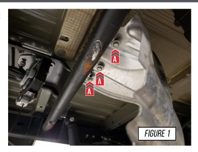
Continue by removing the OE dual exit exhaust by following the steps, shown in **Figure 2**.
