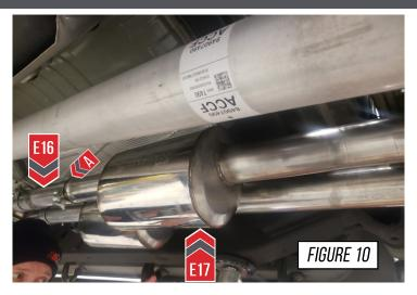
It is crucial to install each section and exhaust band clamps correctly to prevent loose joints, exhaust leaks and rattles.
