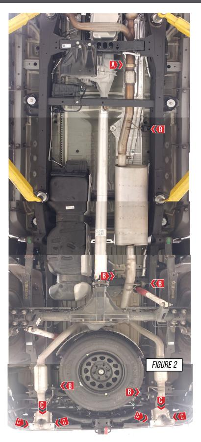
Up next you will need to measure the cut points behind the catalytic converters on the front pipes.
