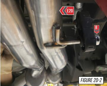
Make your final adjustments to the tips to ensure they are in a position you like. Once the desired positioning is achieved, fully tighten down all clamps.
