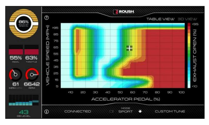
The patent pending Roush Active Exhaust flow control system is unique in the industry and allows the owner of the vehicle to "tune" their exhaust note for their driving conditions and preferences. The Active Exhaust App for iOS gives you the ability to both monitor the Active Exhaust system inside the vehicle while it's operating and design your own custom strategies for deciding how your vehicle sounds. Whether it's on the track or driving through town, you're in control!
