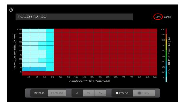
18. With your desired tune selected press "Activate" in order to upload it into the active exhaust module to be stored under the "Custom" setting (this does not affect the touring, sport or track settings).
