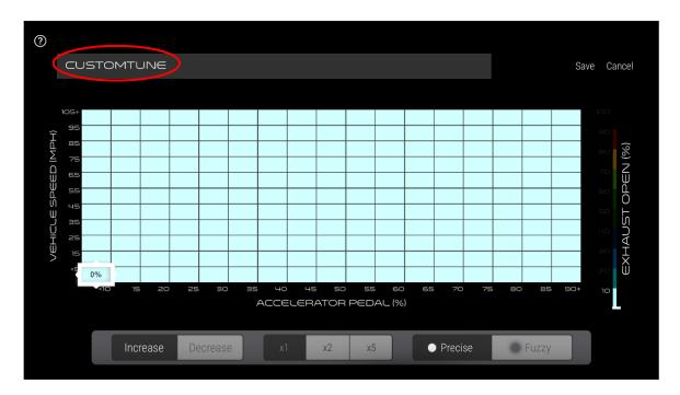
16. Select either increase or decrease, the desired multiplier and either precise or fuzzy to begin shading in the grid. Press and hold on the desired cells to shade them as indicated by the "Exhaust Open (%)" (white means the valve position is fully closed and red means the valve position is fully open).
