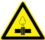
The fuel system is under pressure. Do not open the fuel system until the pressure has been relieved. Refer to the appropriate vehicle service manual for the procedure and precautions for relieving the fuel system pressure.
