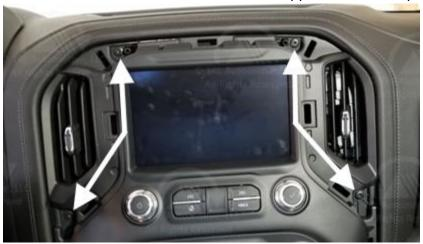
12. Detach the center stack panel. This may require the use of the non-marring pry tool. Be sure to protect prying areas as needed with painter's tape.
