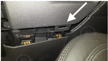
6. Starting from the rear and working toward the front, lift up on the upper console trim panel to detach it. From inside the center console, you'll need to release the clips using a non-marring pry tool.
