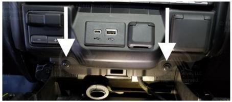
11. Remove the four T15 torx screws from the upper center stack panel.
