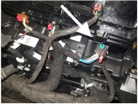
14. **Important**: If bends are required to the Autostop Eliminator wiring, keep pressure between the wire and the connector housings to ensure the wires are not pulled out of the housing. If the wires are accidentally pulled loose from the housing, do not install the device and contact us for a free replacement.
