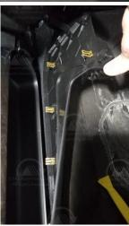
5. Ensure both sides of the lower trim panel are clear from the retainer loop in the upper trim panel.
