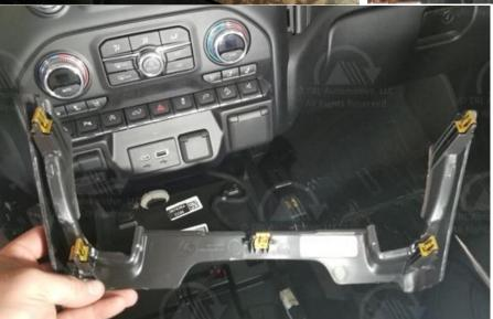
9. Starting from the lower left and working clockwise, remove the upper infotainment trim panel. Unlike the picture below, be sure to use painter's tape to protect any surfaces touched by the non-marring pry tool.
