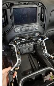
10. Remove both T15 torx screws from the lower center stack panel.
