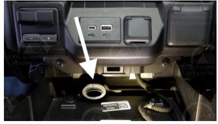
This completes the Autostop Eliminator installation. Please remember that the Autostop Eliminator functions to restore the last state. Assuming OFF is your preference, you may need to press the button once to turn auto stop-start OFF. After that it'll stay OFF.
