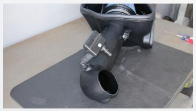
See photo to double check correct installation of vacuum box.
