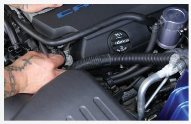
Lift up on the sound tube and move out of the way - then close clip so it can't fall back inside.
