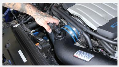
Install the vacuum fitting as shown by simply pushing it into the black grommet.
