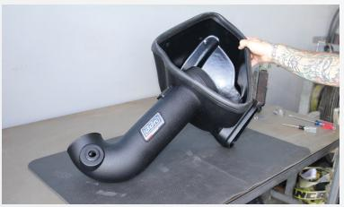
Now turn the inlet tube inside the airbox clockwise to position the tube as shown for the next step.
