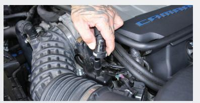
Disconnect the Vacuum line to the left of the MAF as shown by pushing in on the tab from one side at the top and pull up to release. At this time also remove the one time only use clip that secures this black vacuum box to the factory inlet tube (discard the clip - no longer required).
