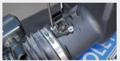
Place the factory airbox and inlet tube assembly on a work bench for disassembly. Start by removing the 2 torx screws that hold the mass air sensor in position. Put the sensor carefully to one side - Do not drop or mishandle put the 2 torx screws back into the factory inlet tube for safe keeping we will not be using them (BBK supplies 2 new screws for the new inlet tube).
