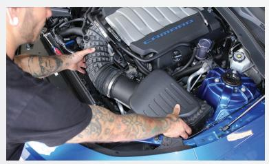
Now is the time to remove the complete airbox assembly - go to the main box and start by pulling it up on each corner to pull it free from the rubber grommet locator mounts.
