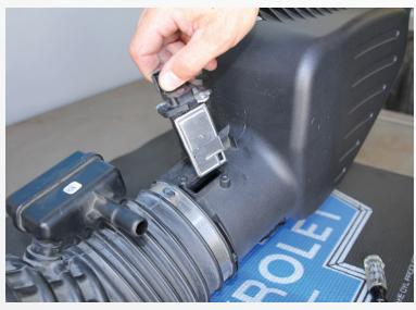
Remove the mass air sensor from the factory inlet tube.
