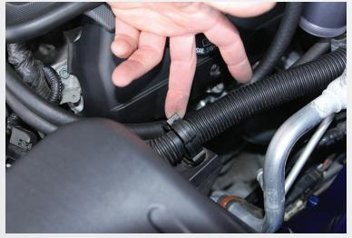
Now move to the drivers side again – the sound tube clip located on the side of the airbox assembly - Lift the tab on the clip and pull apart .
