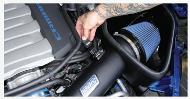
Connect the Mass air wire harness – reverse of number 1 remembering to click the tab back into place to prevent connector from coming loose.
