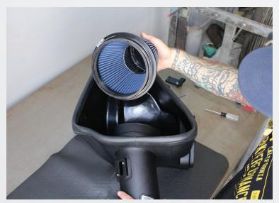
Time to install the air filter - Flat head screwdriver.
