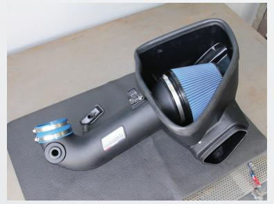
Install the Blue BBK Silicone coupler and clamps as shown - this photo now shows the correct installation of all parts onto the BBK cold air kit.
