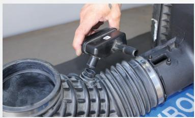
Remove the black vacuum box from the factory inlet tube and place to one side we will be re-using this on the BBK kit.
