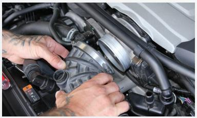
Remove the intake/inlet tube from the throttle body by pulling the tube outwards and away from the throttle body.
