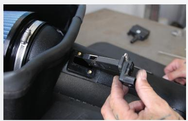
Install the OE Mass Air Sensor - attention: handle the sensor with care - no dirt or oil etc should be allowed to get near - this sensor is directional and will ONLY install one way - the opening/hole at the front of the sensor should be at the front (closest to the air filter as shown in photo).
