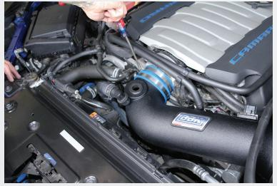
Push the BBK Blue silicone coupler over and onto the Throttle body and tighten the clamps on the air inlet tube and the throttle body.
