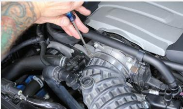
With a flat head screwdriver loosen the clamp that secures the intake tube to the throttle body as shown.
