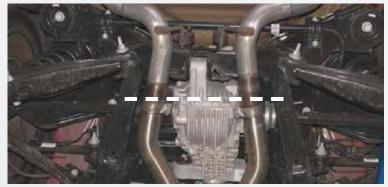
Cut the stock exhaust pipes 1-1/2" forward of where the rear end cover bolts to the third member. Use a sawz-all or air powered cut off wheel to cut the pipes.
