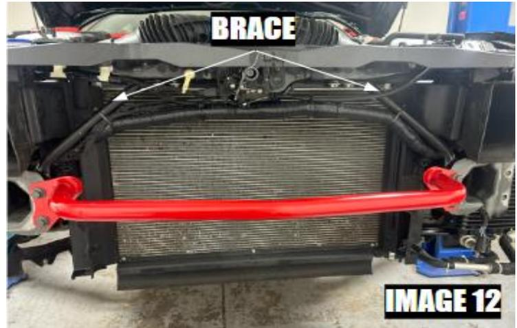
13. Using Zip-ties, secure the wire harness to the bumper support. If your car has the performance package, you can zip-tie the harnessing to the previously mentioned brace
