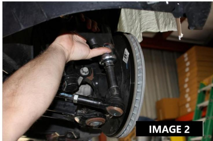
3. Loosen the nut on the outer tie rod end (**IMAGE 2**) and hammer to break the taper free from the spindle
