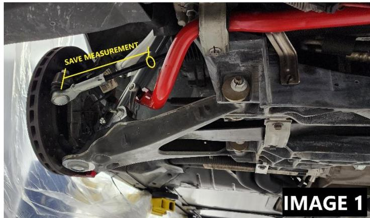
2. Mark a point on the inner tie rod and measure from that point to the centerline of the stud going through the spindle as shown in **IMAGE 1**
