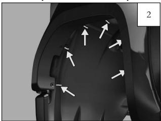
While holding the front flare in place, mark the flare's (6) hole locations using a grease pencil. (Wheel only removed for visual clarity.)
