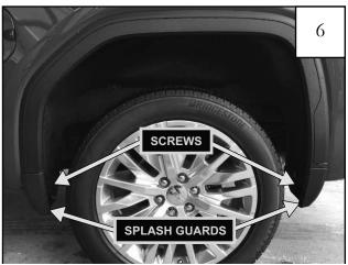
Remove the rear splash guards using a T-15 Torx driver and retain (2) outboard screws for later use.
