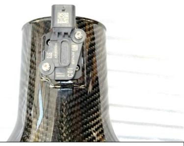
47. Secure the MAF sensor to the carbon housing as shown using the supplied M4 x 12 screws. DO NOT use the stock MAF screws.
