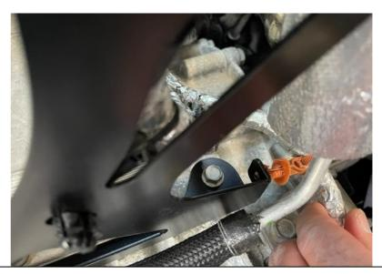
43. The lower wiring harnesses can be secured in the side tabs as shown.
