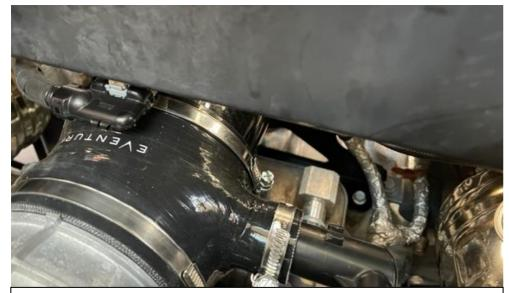
60. Push the MAF sensor plug into the sensor. Make sure it is clicked into place. Secure the hose clamp around the intake. Do not overtighten it – the carbon can get damaged if overtightened.
