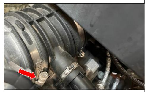
7. Loosen the hose clamp on the rubber inlet hose around the throttle body.
