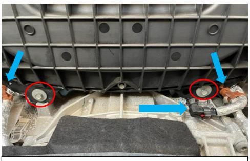
6. Unclip the 2 brown harness attachments from the airbox as well as the temperature sensor. Remove the 2 circled screws. Save these for use later.
