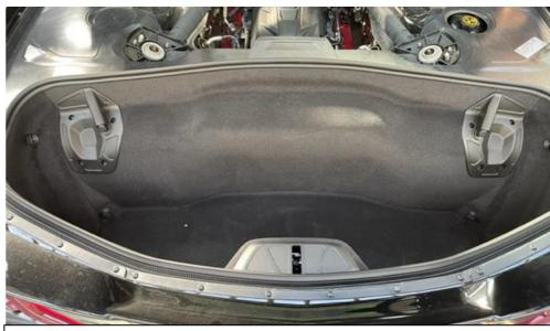
21. Before installing the intake – we will now cut the carpet for the new clear panel. Put just the carpet back into place and secure with the 2 roof mounts on each side.
