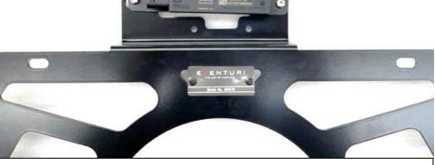
37. Secure the antenna previously removed to the top of the frame as shown using the M4 screws and nuts. The plug side should face the left.
