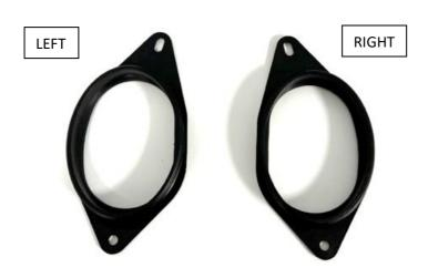
30. Take the new plastic inlet flanges and identify the Left and Right sides. There are L and R markings on the base see next photo.
