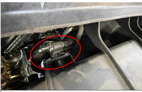
10. At the top of the airbox there are also a couple of plugs which need to be removed on each side.
