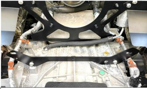
45. Using the stock screws removed previously for the airbox, secure the brace on the remaining mounting points for the airbox as shown.
