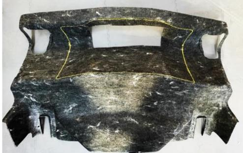
24. With the sides and top marked – mark the base where the carpet folds upwards. The yellow line is what you should have.
