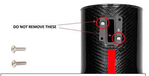
47. Take the supplied M4x12 screws – these will be used to secure the MAF sensor. They may already be screwed into the MAF boss on the carbon housing. If the carbon housing looks like this then the extra screws will be in the kit. **DO NOT remove the screws shown above on the carbon housing. See next step.**
