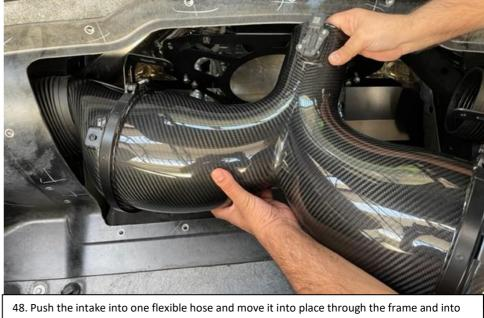
the silicon hose on the throttle body.
