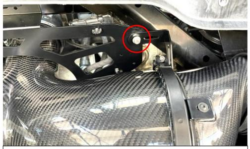
54. Secure the top bracket of the intake to the frame as shown. Do this on both sides. Use the washer at the back before the nut.
