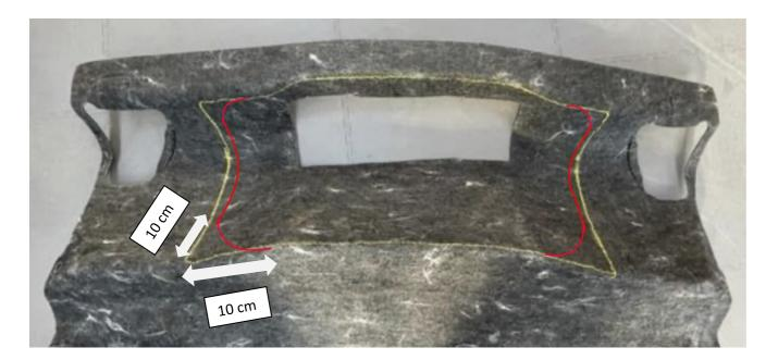
27. The curve at each corner can start 10 cm horizontally and 10cm vertically from the corners as shown. Each one can be the same.
