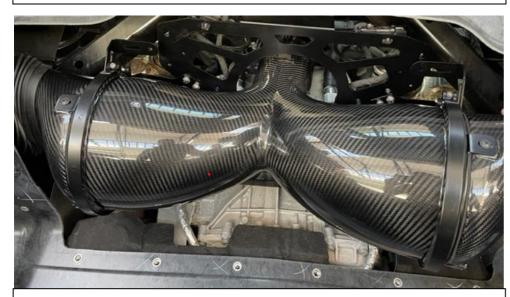
49. Push it into the silicon at the throttle body – make sure the clamp around the silicon is loose. As you move it into place – get someone to pull the other flexible hose on the side. You could also manipulate the flexible hose into position yourself after getting the intake into place.
