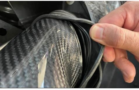
51. Pull the flexible hoses over the intake on both sides. Ensure the hoses are fully latched onto the carbon. No clamps are required.
