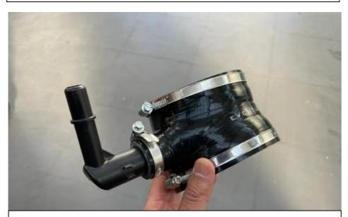
19. Take the new silicon hose and insert the plastic breather elbow into the side opening. Push it in as far as possible. Leave the hose clamps loose for now.
