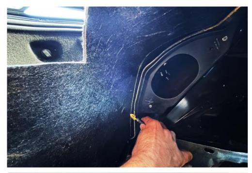
23. Using a crayon (or similar) mark the opening around the sides and top of the carpet from the inside. Use the factory opening as the template.
