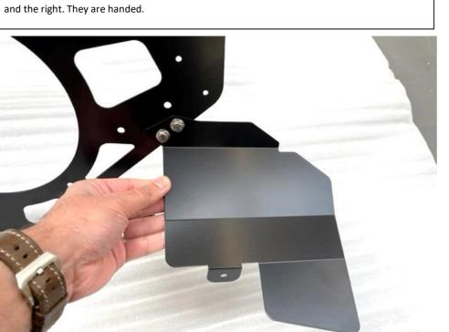
36. Secure the shields to the frame using the holes shown.
