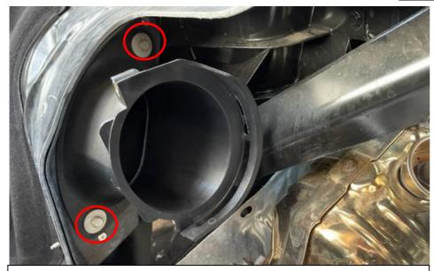
20. Remove the 2 side inlets by unscrewing the screws as shown.
