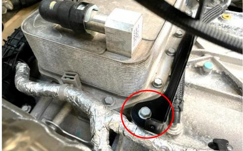
39. Use the stock screws previously removed to mount the frame as shown on both side.
