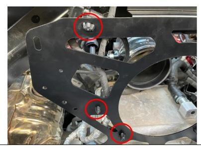
40. Clip the wiring harnesses into the frame. Shown without the shields for clarity. Do the same for both sides.
