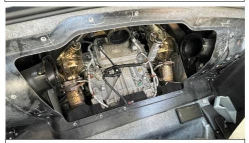
15. Airbox can be completely removed.
