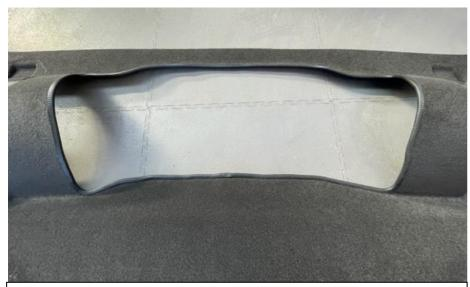
28. Cut out the shape marked by the red lines on the sides and the yellow lines on the top and bottom – then using the supplied edging, push it onto the exposed carpet. Start from the bottom in the middle and work your way around.
