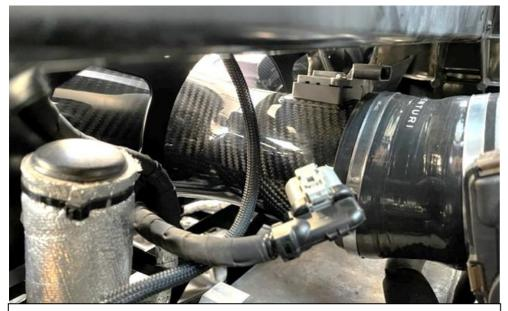
50. Ensure that the intake goes squarely into the silicon as far into it as possible. Make sure the silicon is not pinched anywhere.
