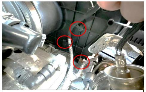
9. There are a number of clips which need to be removed from the airbox on the engine side.
