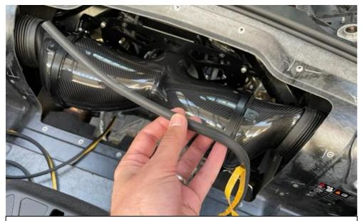
62. Take the supplied self adhesive rubber sealing strip and remove the backing to expose the adhesion.
