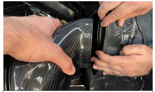
Illustration of the flexible hose being pulled back while the intake is moved into position.
