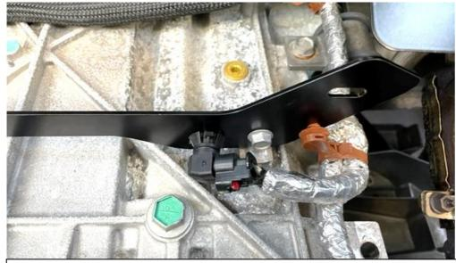
46. Push the temperature sensor into place and also the wiring harness as shown – on both sides.
