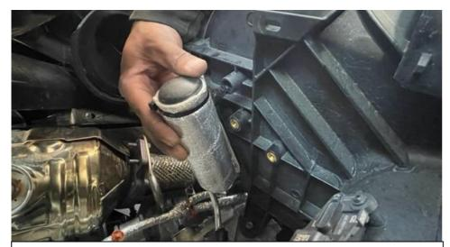
13. The airbox can now be pulled out to gain more access to the back. This insulated module can be removed from the airbox either by prising the clip out or by disconnecting the rubber hose at the base of it from the gearbox and then unscrewing it from the airbox once the airbox is completely removed.
