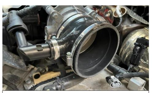
19b. Install the silicon hose onto the throttle body and push the breather elbow into the clip again. It will click into place. Make sure the silicon is fully pushed onto the throttle body. It should be flush on the inside all around. Now secure the clamp around the throttle body and the breather.
