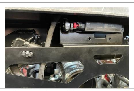
42. Push the antenna plug into the antenna and lock with the tab.
