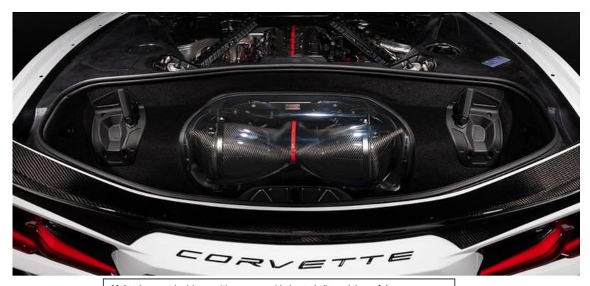
66. Put the carpet back into position – secure with the stock clips and the roof clamps.
