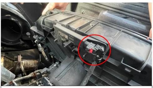
14. Disconnect the plug from the sensor at the top of the airbox.
