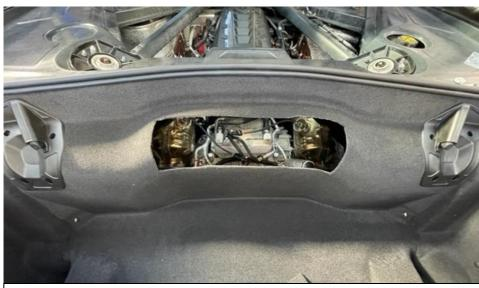
22. Using a sharp utility knife, make an access hole in the middle of the carpet. This will allow you to mark the inside.
