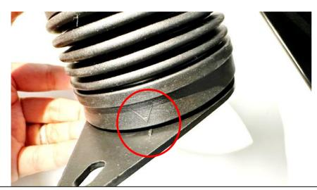
32. Push the provided flexible hoses onto the inlets. Line up the V logo on the hose to the mark on the inlet as shown. Clamps are not required. Make sure the hose is pushed down evenly all around. The Top of the hose has "C8 Filter Side" marking on it.
