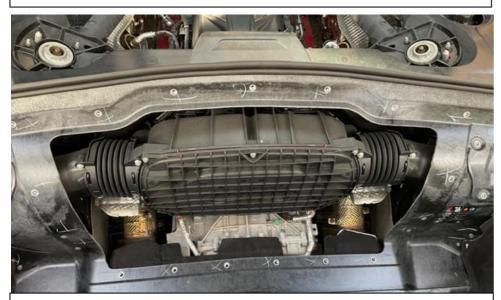
3. With the panel removed we can now start to remove the airbox.
