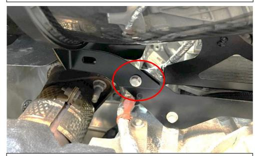
56. Using another M6 screw and nut (no washer required), Secure the lower intake bracket to the brace installed previously. Do the same on both sides.
