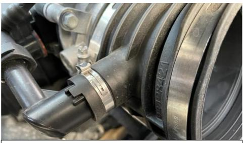
18. Remove the rubber hose from the throttle body and then remove the plastic breather elbow from the hose.
