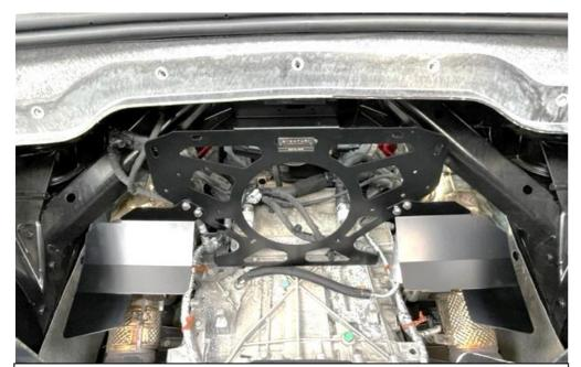
38. Install the frame as shown – it will mount to the stock airbox mounting positions – see next photo.
