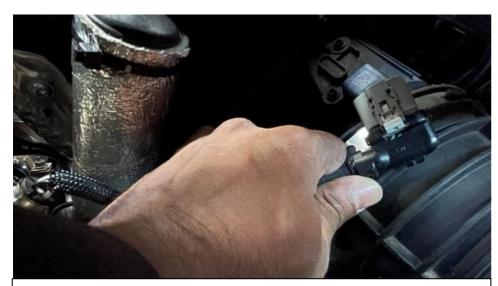
11. Unclip the MAF sensor plug from the back of the airbox.
