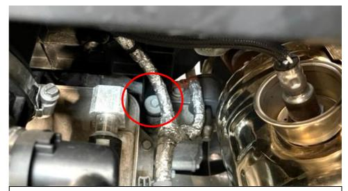
12. Remove the 2 screws holding the airbox down on the engine side. One of them is circled in the above photo. There is another on the other side. Save these for use later.
