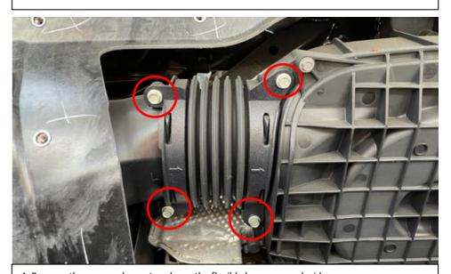
4. Remove the screws shown to release the flexible hoses on each side.
