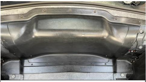
2. Now remove the screws holding the trunk panel in place. We will re-use these screws for the new panel.
