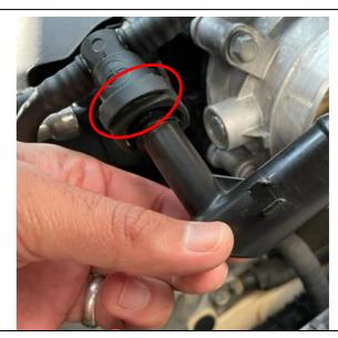
8. Depress the clip as shown and pull the breather pipe out from the connecting clip.
