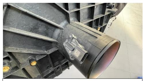
16. Remove the MAF sensor from the airbox. We use new screws to secure it to the intake.
