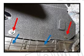
Remove 2 x 7mm screws and pull panel down. The led strip will mount on these 2 ribs (blue arrows)
