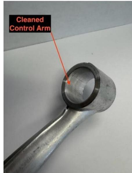
15. Before installing the new control arm bearings, clean the control arm with brake parts cleaner to remove any remaining debris from the old bushings.
