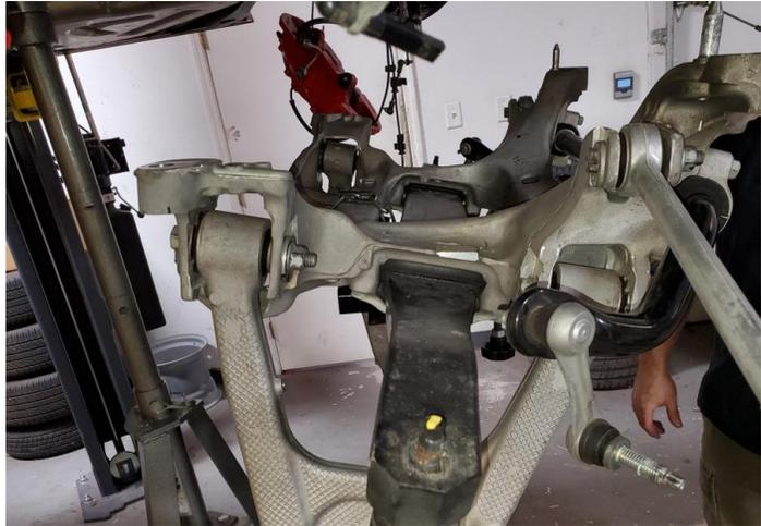
18. After removing the rear lower control arm, the rear cradle can be raised and reinstalled.
