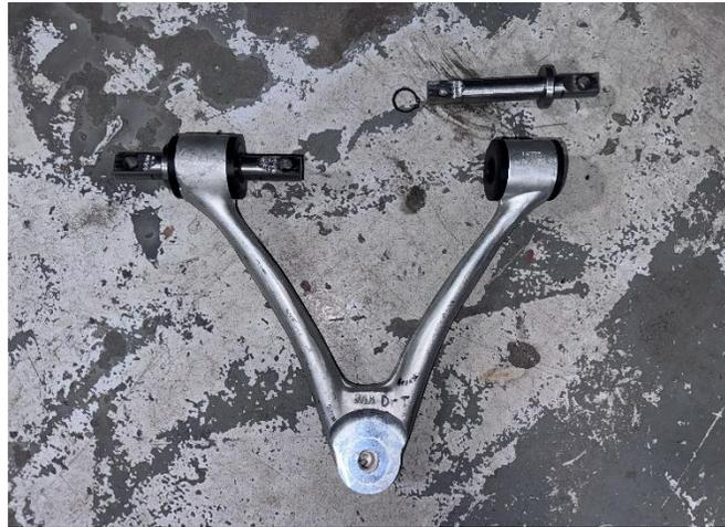
39. Install the control arms back into the car and assemble all other components taken off during installation.
