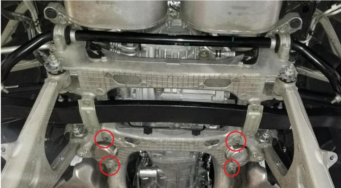
14. Remove the four (4) nuts from the transmission mounts as shown.
