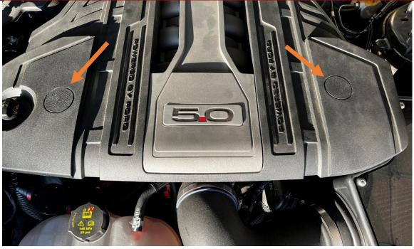
1. Remove engine cover by using a flathead screwdriver to remove the caps, revealing the bolt and nuts. Use a 10mm wrench to remove the nuts. Once nuts are removed, pull the engine cover off the 4 mounting points to remove the cover from the vehicle.
