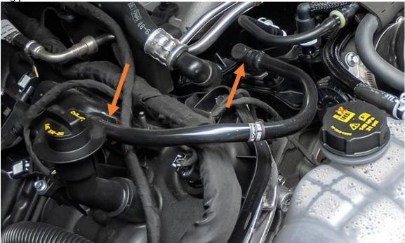
2. Remove stock PCV Line from vehicle by pulling on the tab on the 2 quick disconnect fittings.
