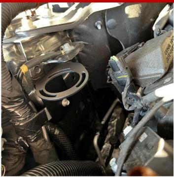
Use an 8mm Wrench to remove the bolt located next to the passenger side shock tower. Insert the Catch Can bracket and reinstall the 8mm bolt to secure bracket.
