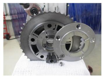
**Step 8:** Place **anti-seize or high-pressure lubricant** on the pipe plug, and thread the plug into the lock. Use your 5/32" Allen socket or wrench to tighten the plug until the lock does not move.
