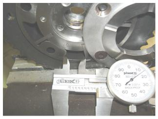
Other cam phasers have ~.815 in. chamber width (52 crank deg.)
