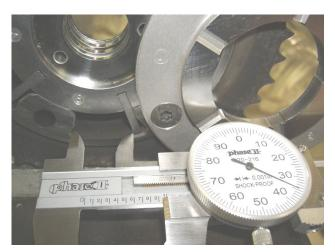
LT4 cam phasers have ~.935 in. chamber width (62 crank deg.)
