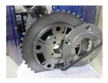
**Step 9:** Rotate the cover plate back over the control chambers and reinstall the safety bolt. Reinstall the cam phaser bolts, making sure to install the pin-bolt back into the correct position. Remember to torque the bolts to 85 in. lbs.
