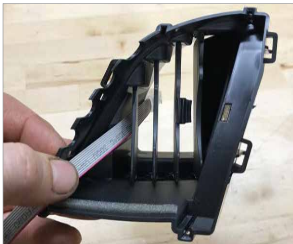
6 Feed display cable through vent as shown.
