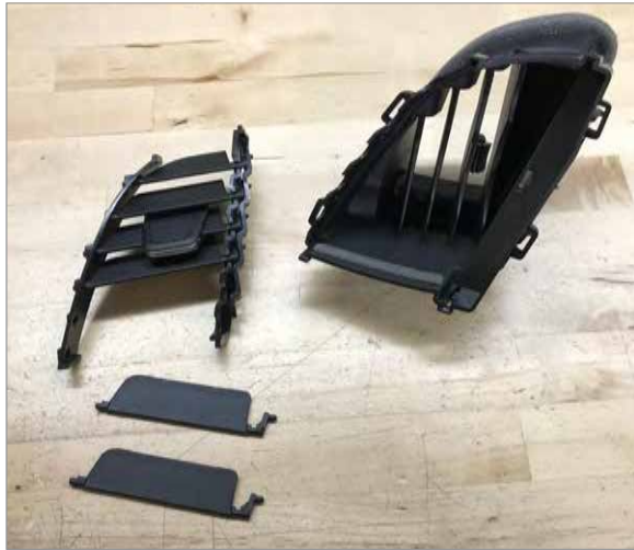
3 Remove bottom two vent slats from assembly.
