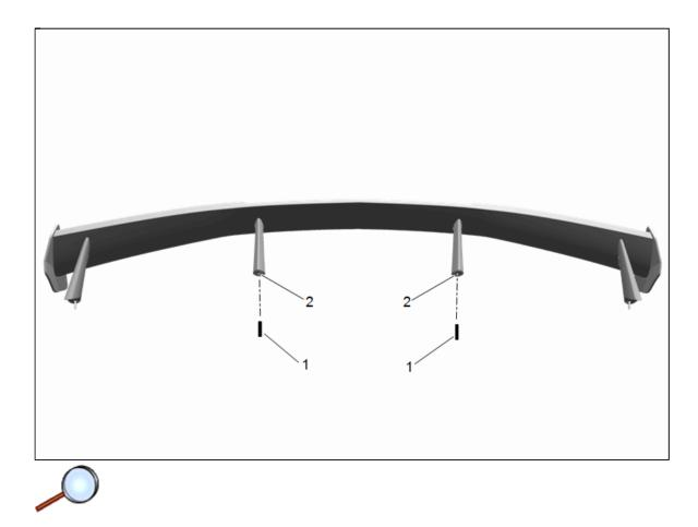
1. Insert the temporary locating pins (1) into the inboard stanchions (2) of spoiler.
