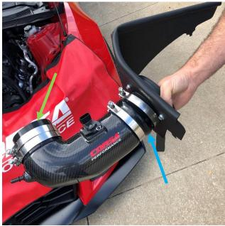
5. Attach Silicone Hose (#5) and 4" T-Bolt Clamps (#6) to throttle body side of air duct. Attach Silicone Hump Hose (#8) and 4.375" T-Bolt Clamps (#7) to opposite end of air duct. Slide Silicone Hump Hose over the Filter Adaptor.
