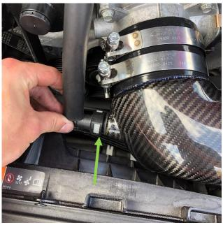
6. You can now insert the CORSA air intake into the engine bay. Make sure the Aluminum Heat Shield sits in the 3 rubber grommets from Step 8 of removal instructions. Connect breather hose to air duct using the Connector Fitting.
