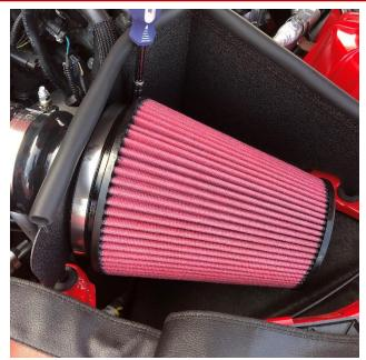
**9.** Attach the Air Filter (#3) to the filter adaptor so it sits inside the heat shield. Tighten the clamp using the 8mm socket as shown.
