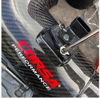
Install factory MAF sensor to the air duct using the 2 provided screws (#13) and a Phillips screwdriver.
