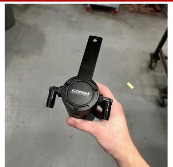
Install barbed fittings and bracket to the catch can using an 11/16" wrench and 2.5mm Hex wrench. IMPORTANT: Corsa recommends using thread sealant or PTFE tape on barbed fittings and bottom drain plug to prevent any leaks.
