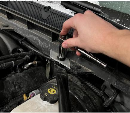
**3.** Remove bolt on driver's side strut brace above the coolant reservoir using a 13mm wrench. Place catch can bracket on top of flat surface and reinstall bolt.
