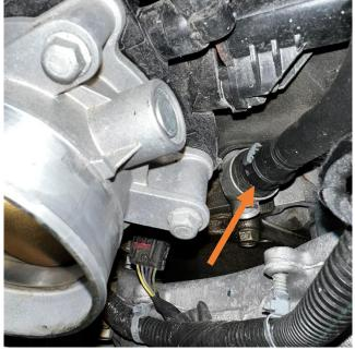
2. Remove stock PCV line which is located underneath the throttle body on the driver's side of the vehicle.
