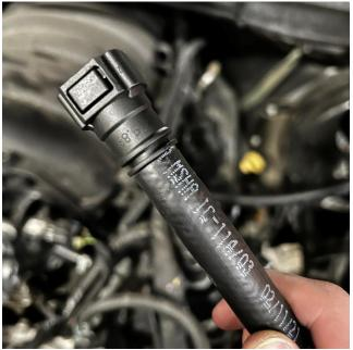
2. Attach quick disconnect fittings to one end of each of the provided hoses. A mild lubricant or heat may be needed to fully install fitting into hose.
