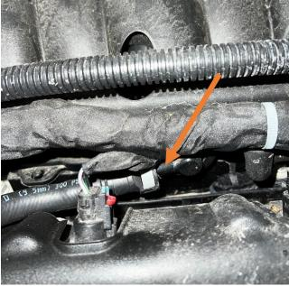
**3.** Remove other end of PCV line located underneath the intake manifold on the driver's side of the vehicle.
