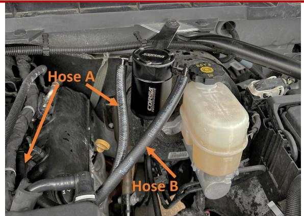
4. Hose A to the "A" side of the catch can and route it to the fitting located underneath the intake manifold. Connect Hose B to the "B" side of the catch can and route the line to the fitting located next to the throttle body. Make sure all quick connect fittings are secured in place and hose is pushed all the way over the barbed ends of the fittings. Reinstall air intake.
