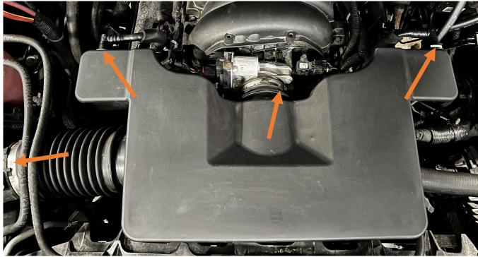
1. Remove air intake by loosening the clamp on the throttle body and the clamp on the airbox using an 8mm socket. Unclip the two quick disconnect fittings in the top right and left corners of the intake by pressing on the grey tabs and pulling.
