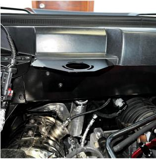
Locate the two bolt holes next to the passenger side shock tower. Use the provided hex bolts and a 4mm Allen Wrench to secure the bracket in place.
