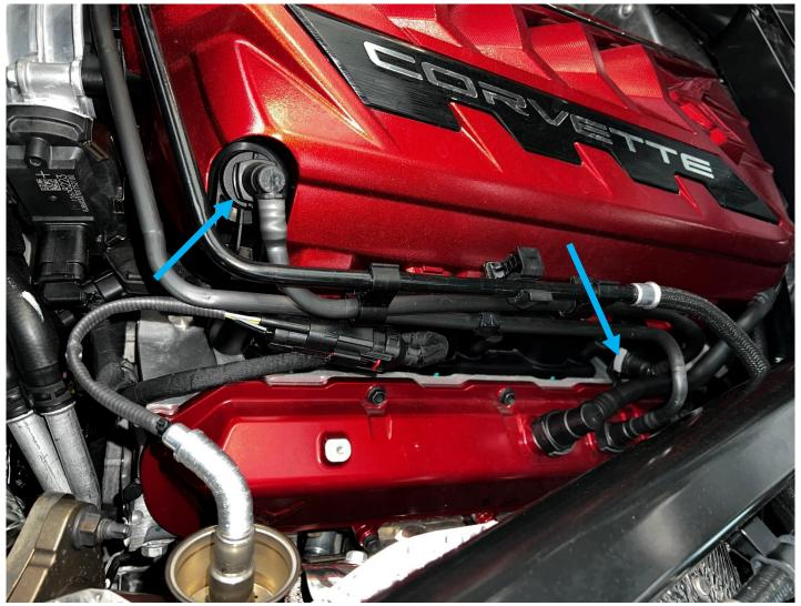
1. Locate and remove stock PCV line from the passenger side of the vehicle by pressing on the grey tabs and then pulling on the quick disconnect fittings. Detach the PCV line from the 2 wiring harness clips.
