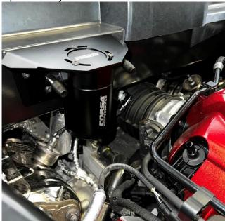
**3.** Attach the can to the bracket using the 3 hex bolts located on top of the catch can. Use a 2.5mm Allen Wrench to tighten down bolts.
