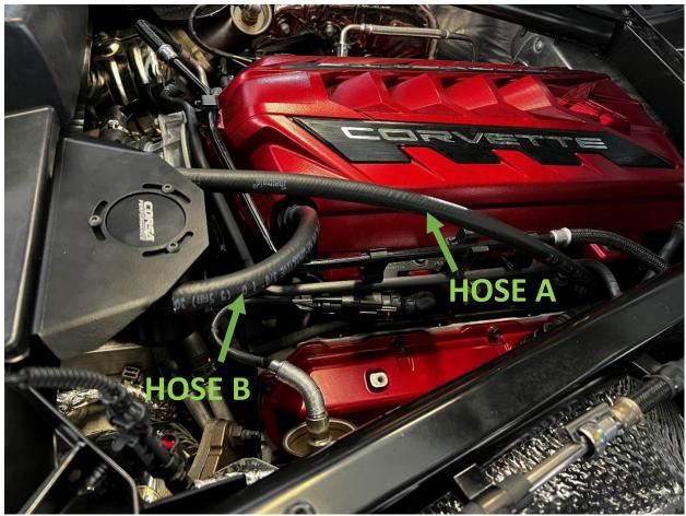
5. Install Hose A to the "A" side of the catch can and route it to the engine fitting located closest to the front of the vehicle. Route hose B from the "B" side of the catch can to the fitting coming out from the engine cover. Make sure all fittings are secured in place and hose is pushed all the way over the barbed ends of the fittings.
