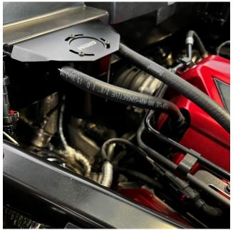
**4.** Insert the straight quick disconnect fitting to Hose B and the 45 degree elbow quick disconnect fitting to Hose A. **NOTE:** Installing fittings to hose may require heat or lubrication.
