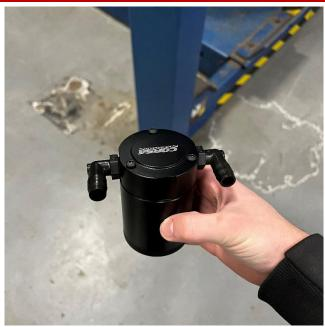
Install 3/8" NPT fittings to catch can using an 11/16" wrench. IMPORTANT: Corsa recommends using thread sealant or PTFE tape on barbed fittings and bottom drain plug to prevent any leaks.
