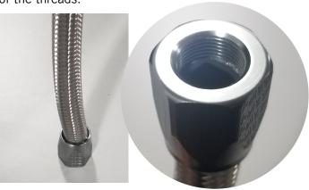
4 Place some grease on the fitting on the hose end before threading it into the nut. This will prevent it from biting the hose and tearing it.
