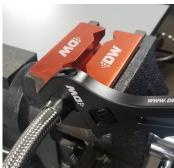
**7** Make sure the nut is well secured and tight. Lining up the hex on the nut and the hose end is a nice touch, as later on in the vehicle it makes for sliding on a wrench that much easier. The picture below it what the finished product should look like. As with all fuel system components, double check for any leaks before driving the vehicle.
