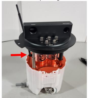
8 – Attach the remaining smaller 1/8-inch end of the venturi hose to the 1/8-inch hose barb fitting on the underside of the hat, and secure with the provided 6mm hose clamp.
