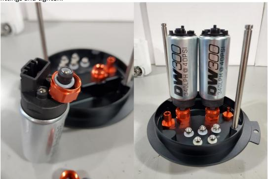
2 – Install the supplied 3/8" convoluted tube onto the return fitting and secure with the supplied 3/8" pinch clamp. Slide the center plate over the pumps and return tube, reinstall the e-clips, cut the return hose flush with the bottom of the return plate when its fully extended.
