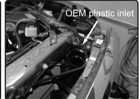
4. Locate the plastic intake inlet, remove the push clip and lift up but do not remove. This will allow the removal of the air box.
