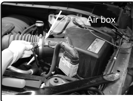
5. Disconnect the MAF sensor harness.
