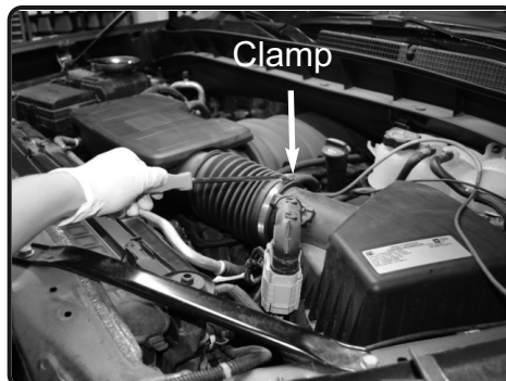
6. Loosen the clamp on the air box using 8mm nut driver.
