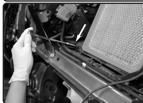
11. Loosen the bolt holding in the lower part of the air box using 10mm socket and ratchet. Save for later install.
