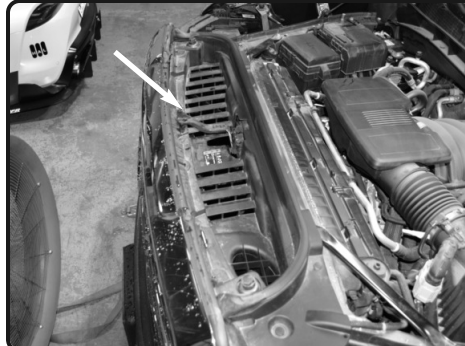
2. Loosen and the nut holding in the hood latch and remove.
