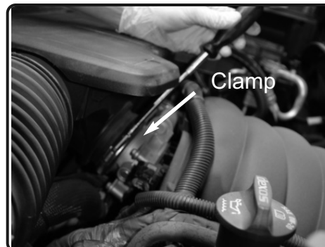
7. Loosen the clamp on the throttle body using 8mm nut driver.
