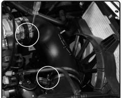
**21.** Now secure and tighten all clamps using 8mm nut driver.
