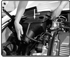
**17.** Install the airbox assembly to the factory position.
