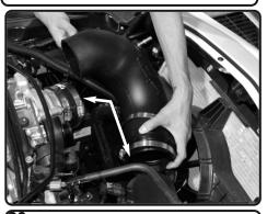
**20.** Install the intake tube. Attach the with clamps to the intake tube. Position for best fit.
