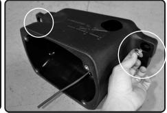
11. Now install the grommets and washer-spacers to the new injen airbox.
