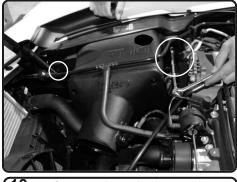
**18.** Secure the air box using factory bolts. Tighten and secure using 10mm socket and ratchet.
