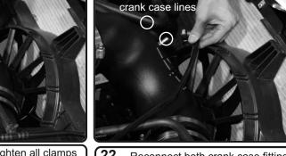
**22.** Reconnect both crank case fittings. Some models only have 1 crank case line. Remove the fitting and use the supplied 3/8"-16 Hex bolt to block the fitting if not used. Secure threads with Loctite
