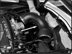
**4.** Now pull out the intake tube out of vehicle.
