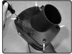
**15.** Place the Injen plenum onto the Injen lower air box assembly and use 4-M6X20 bolts and rubberized washers secure the plenum to the lower air box.
