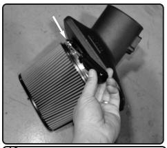
**13.** Place the filter onto the Injen plenum and then secure the clamp
