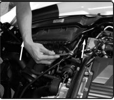
**6.** Loosen the two 10mm bolts holding in air box.
