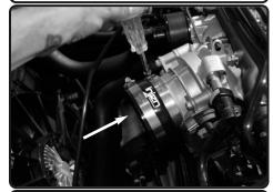
**9.** Install the straight hose with clamps to throttle body. Tighten the clamp on throttle body only.
