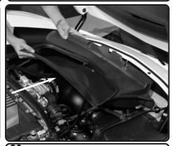
**23.** Re-install air vent and secure.
