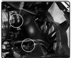
**10.** Now secure and tighten all clamps using 8mm nut driver.
