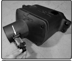
**5.** Now install the MAF sensor into the plenum. Secure using provided M4 screws.
