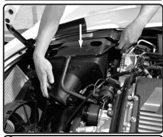
**6.** Install the airbox assembly to the factory position.
