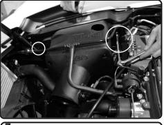
7. Secure the air box using factory bolts. Tighten and secure using 10mm socket and ratchet.
