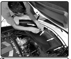
**2.** Use a 7mm nut driver to remove the four air vent screws. Remove the air vent from the engine bay for now.
