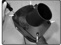
**3.** Place the Injen plenum onto the Injen lower air box assembly and use 4-M6X20 bolts and rubberized washers secure the plenum to the lower air box.
