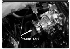
**9.** Install the 4" hump hose with clamps to throttle body. Tighten the clamp on throttle body only.
