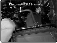
**5.** Pull back lines away from the air box. Disconnect MAF sensor harness.
