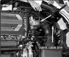
**3.** Loosen the clamps on the stock intake tube using 8mm nut driver. Disconnect the crank case line on intake tube.
