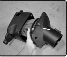
**14.** Install the plenum assembly into the lower air box.
