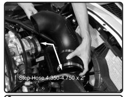
**9.** Install the intake tube. Attach the step hose with clamps to the intake tube. Position for best fit.
