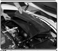
**12.** Re-install air vent and secure.
