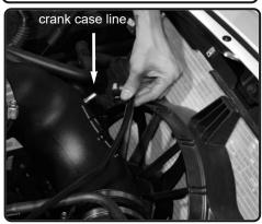
11. Re-connect the crank case fitting.
