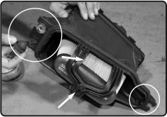
**10.** Remove the ractory grommets and washer-spacer out of air box. These will be used on new injen air box. Keep same finguration.
