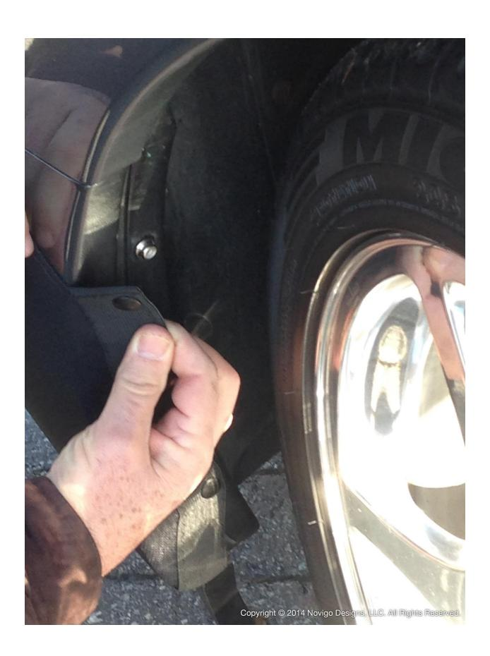
Begin the installation by fastening the snaps on one end of the mask to the screws just installed on the edge of the bumper.
