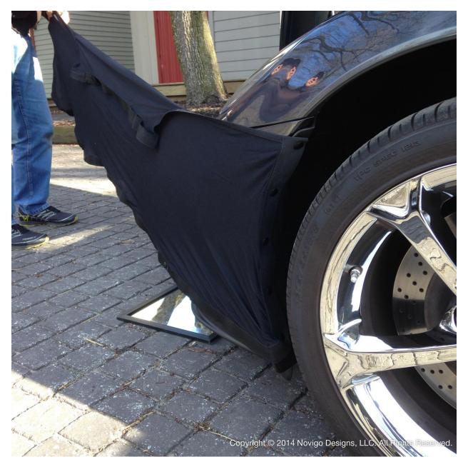
Stretch the mask across the front of the bumper and attach to the other side of the car. **Note**: the tension in the mask is normal and important to the overall performance of the product.
