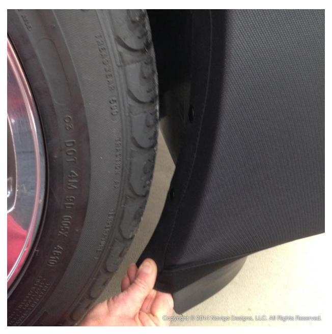
Locate and slightly loosen the screw holding the corner of the air dam on each side of the car allowing the bottom edge of the mask to go between the bumper and the air dam. **Note**: Do not install mask over the air-dam.
