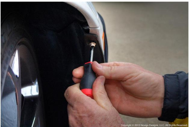
Locate the mounting pins at the edge of the bumper inside the fender liner and remove the four (4) pins that attach the fender liner to the front bumper starting with the top pin.
