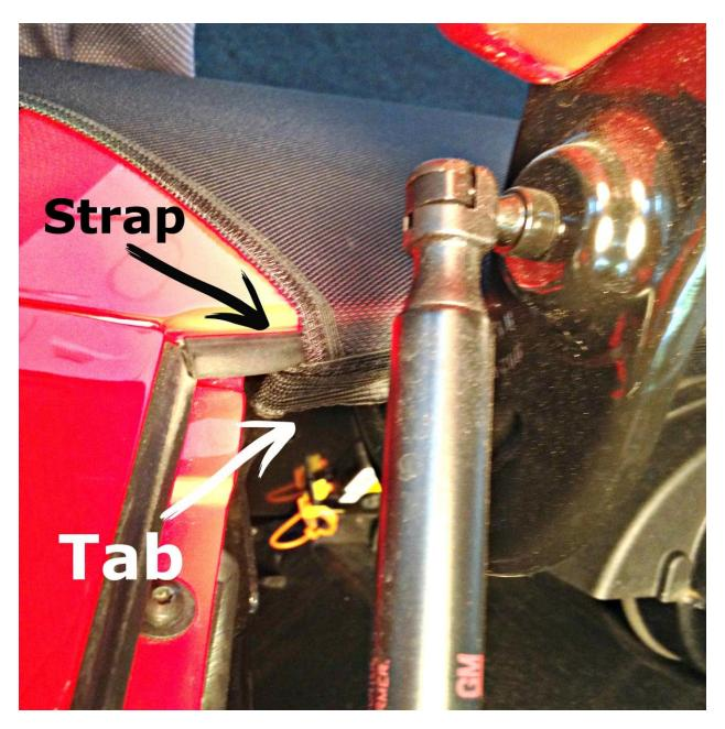
Open the hood. Hold the top of the mask and pull it up to the hood opening. Secure the top corners of the mask to the body frame by looping the open straps on the mask over the tab alongside the hood-hinge.
