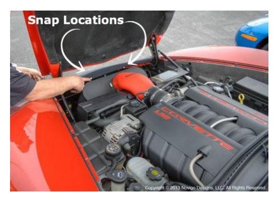
Remove the screws on the frame that best align with the snaps on the mask and replace with a snap-head screw stud. Secure the mask by fastening the snaps on the mask to the snaps just installed.
