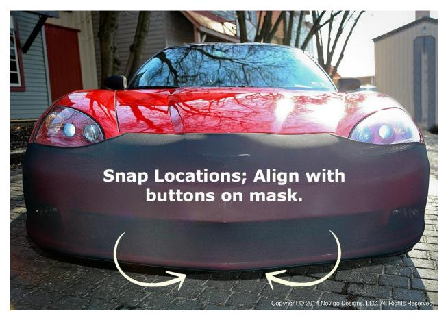
Pull the bottom edge of the mask down under the bumper, noting the position of the snaps on the bottom edge of the mask. Replace the screws on the bottom of the bumper that best align with the snaps on the mask with a snap head screw stud. **Note**: the screws on the bottom of the C6 are approximately 10" back front the front edge of the bumper in slightly recessed wells and can be easy to overlook. Fasten the snaps on bottom of the mask to the screws just installed on the bottom of the bumper.
