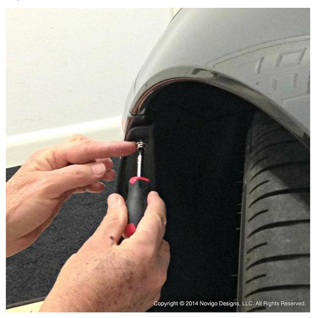
Locate the mounting screws at the edge of the bumper inside the fender liner and remove them. Replace each one as you go with the supplied snap-head screw studs. Repeat this step on the other side of the car.
