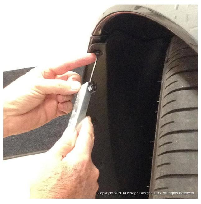
Turn the front wheels to gain easier access to the fender liner mounting screws that you will be replacing.
