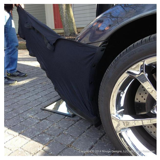
Stretch the mask across the front of the bumper and attach to the other side of the car. **Note**: Take extra-care when stretching the mask over and around the Splitter or Spoiler, rough edges and corners on ground fx can damage the mask over repeated installations.
