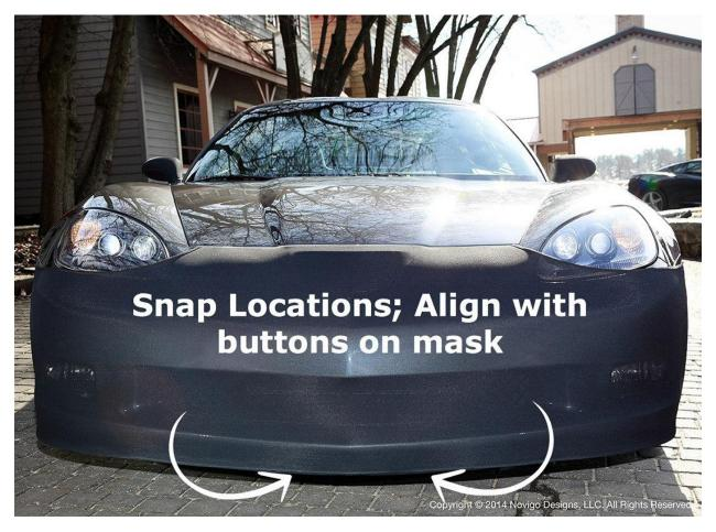
Pull the bottom edge of the mask down under the bumper, noting the position of the snaps on the bottom edge of the mask. Replace the screws on the bottom of the bumper that best align with the snaps on the mask with a snap head screw stud. Fasten the snaps on bottom of the mask to the screws just installed on the bottom of the bumper.
