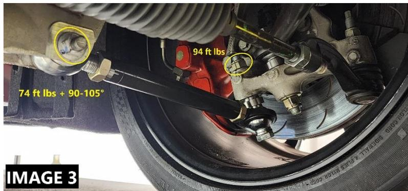
7. Use the supplied nut and bolt to fasten the tapered stud to the spindle. Torque to **94 ft lbs** **IMAGE 3**
