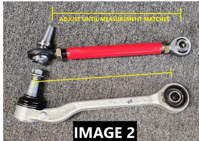
5. Lock down the jam nuts by holding the body of the rod end and tightening the jam nuts to the threaded tube using a **1-1/8"** wrench, and position the arm in the vehicle.
