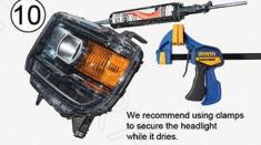
Remove any old sealant still in the lens groove. Reseal the headlight by forming a solid bead of RTV silicone adhesive. We suggest using ORACLE Headlight Sealant. Allow enough time for the sealant
