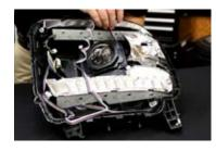
7. Run the RGBW ribbon cable out of headlamp, sealing any hole that you may create. Replace the headlamp lens and repeat for the other side.
