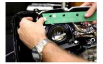
1. Remove the headlamp lens. Using a T20 Torx Screw Driver, remove the screws holding both reflector housings in place to access the factory LED panels. Pull the reflector housings away from the headlamp and unclip each connector.
