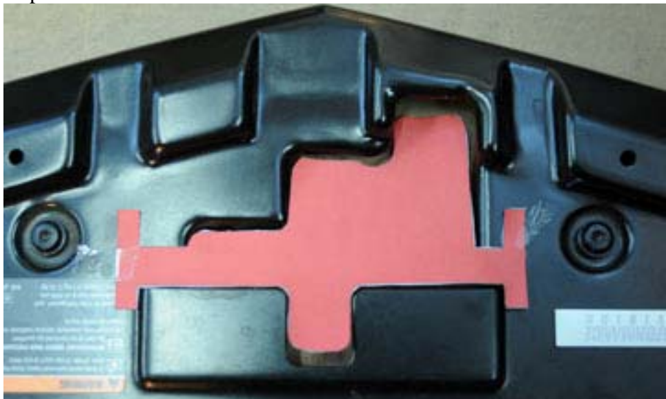
16. Cutout and attach template on last page of instructions to radiator cover panel and cutout to match template.
