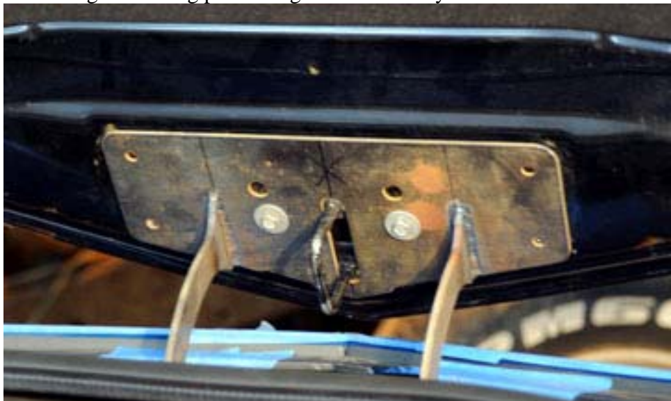
20. Bolt Hood to hinge mounting plate using 2 center factory bolts
