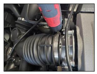
Locate the clamp securing the stock Air Duct to the Throttle Body and loosen with an 8mm Socket & Ratchet or Nut Driver.
