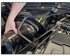
11. After ensuring the Gasket is in place on the CORSA Carbon Fiber Air Box opening, carefully insert the CORSA Carbon Fiber Air Duct and Filter into the Air Box. Double check the Gasket between the Air Box and Air Duct is not pushed into the Air Box. When fully installed, the Filter and Clamp will not be visible.
