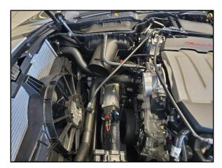
Carefully remove the stock Air Duct.
