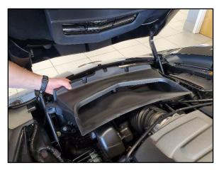
Carefully remove the Radiator Air Outlet Duct and with the 4 Screws, set aside in a safe place. This will be reinstalled on Installation Step 16.
