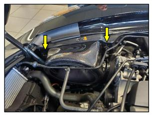
**4.** Install the 2 stock Mounting Bolts with a 10mm Socket & Ratchet or Nut Driver and torque to 80 in-lbs (9 N-m).
