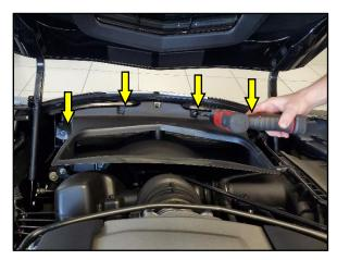
Locate and remove the 4 Screws securing the Radiator Air Outlet Duct with a 7mm Socket & Ratchet or Nut Driver.
