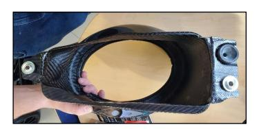
Assemble the 3 stock Mount Hardware into the CORSA Carbon Fiber Air Box in the same orientation and position as stock.
