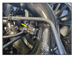
13. Locate the MAF Sensor Harness and push Plug onto the MAF Sensor. Push the RED Clip down on MAF Sensor Plug to lock it in place.
