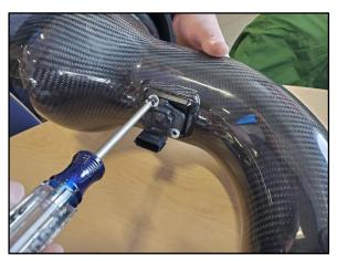
Insert the MAF Sensor into the CORSA Carbon Fiber Air Duct. Install the included black MAF Screws, using a #2 Philips screwdriver and torque to 35 in-lbs (4 N-m).
