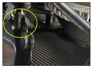
Install the CORSA Carbon Fiber Air Box by first pushing the Lower Rear Mount onto the Stud on the Fender
