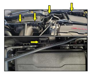
**8.** Carefully remove the Surge Tank Coolant Hose from the 2 Hose Retainers on stock Air Box, Hose Retainer on the Fender, and the Hose Retainer between the Fuse Box Cover and Fender.
