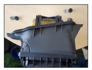
Note the orientation and position of the 3 stock Mount Hardware and then carefully remove them from the stock Air Box. These will be reused.
