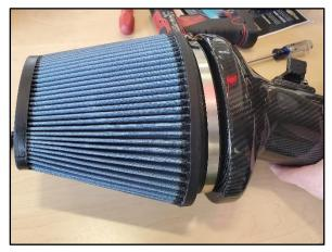
10. Ensure the Clamp is seated on the Air Filter, then Slide the Filter and Clamp onto the CORSA Carbon Fiber Air Duct. Using an 8mm Socket & Ratchet or Nut Driver, torque the Clamp to 44 in-lbs (5 N-m).
