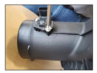
Locate the stock Air Box, then locate and remove the 2 MAF Screws. The screws will NOT be reused.
