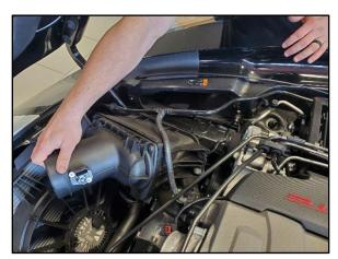
10. Carefully pull on the stock Air Box to release the remaining Mount and remove it from the vehicle. Ensure all the Mounting Hardware is in place on the stock Air Box. This will be needed in Installation Step 1.
