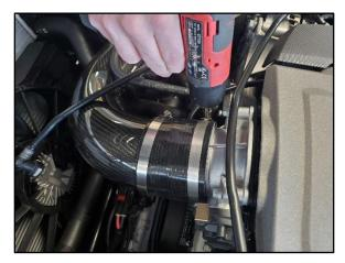
12. Insert the Silicone Sleeve onto the CORSA Carbon Fiber Air Duct, then slide the 2 Clamps over the Silicon Sleeve. Next, insert the Silicon Sleeve onto the Throttle Body. Using an 8mm Socket & Ratchet or Nut Driver, torque the Hose Clamps to 44 in-lbs (5 N-m).
