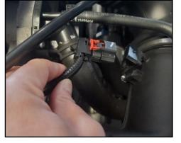
3. Locate the MAF Sensor on the Stock Air Duct. Pull the RED Clip on MAF Sensor Plug. Squeeze the Black Tabs under RED Clip to release the Plug then pull the Harness from the MAF Sensor. Move the Wiring Harness out of the way for now.
