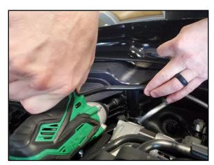
Locate and remove the 2 screws securing the stock Air Box to the Fender with a 10mm Socket & Ratchet or Nut Driver.
