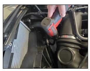
6. Locate the clamp securing stock Air Duct to the stock Air Box and loosen with an 8mm Socket & Ratchet or Nut Driver.
