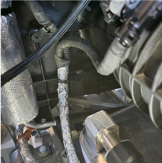
16. Cut the cable tie for the canister mounted to the air box.
