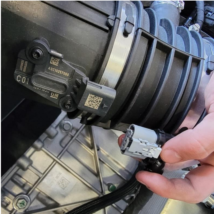
18. Unclip the wiring harness from the MAF sensor.
