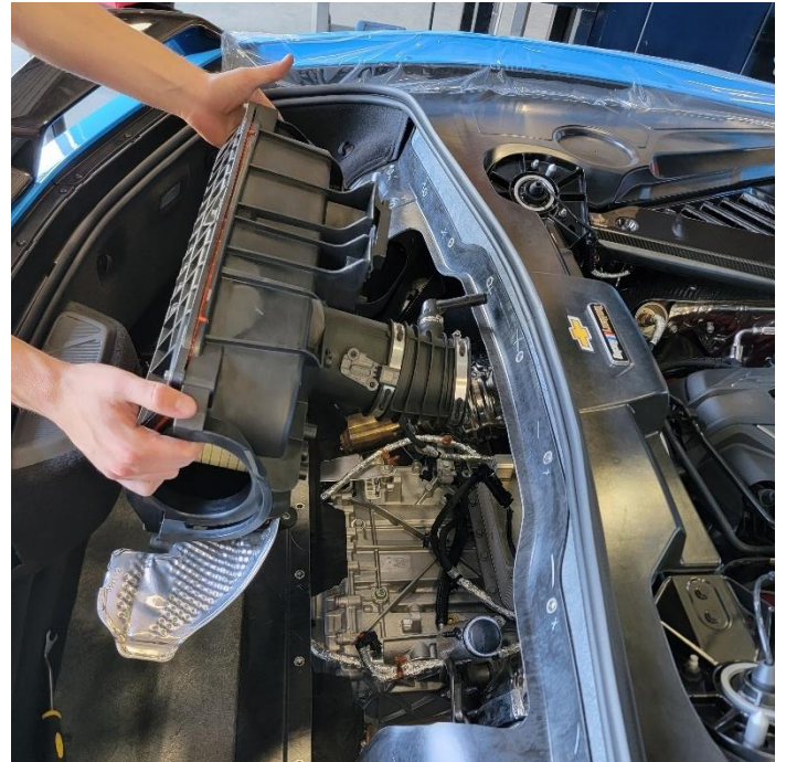
19. Remove the air box assembly from the vehicle.
