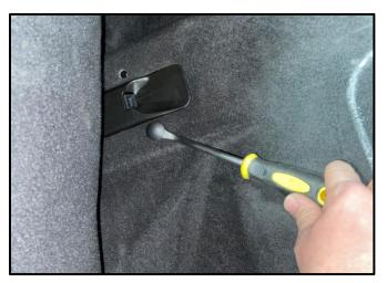
Using an Trim Removal Tool or similar, remove the Push Pin Fasteners. There are 2 on each side. located at the back of the Vehicle's trunk floor.
