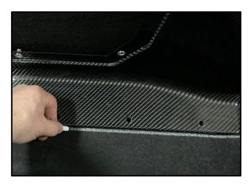
3. Using a piece of Chalk or a similar NONpermanent method of marking, draw an outline around the entire CORSA Carbon Fiber Trunk Panel onto the Trunk Carpet.
