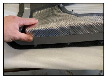
22. Next, bend the Heat Shield over to the edge of the Gasket. DO NOT OVERLAP the Heat Shield and the Gasket. Gently press the Heat Shield against the Carbon Panel, starting at the Gasket. The Heat shield may form a wrinkle and stick to itself going over the radius. This will not affect the performance of the Heat Shield.
