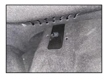
Once satisfied with the Trunk Carpet cutting, locate and reinstall the Push Pin Fasteners from Step 7 and tighten the screws for the Roof Storage Latches.
