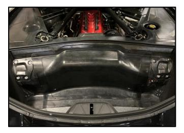
Remove the Net Attachment Clip-Nuts from the lower front corners of the trunk by unscrewing them.
