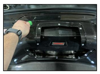
23. Locate the Trunk Panel Screws from Step 9. Starting with the Top Center Screw, loosley start all 19 screws, using a T15 Torx Driver and ONLY BY HAND.
