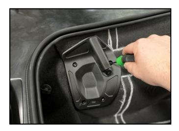
Using a T15 Torx Driver, remove the 4 screws from both Factory Roof Storage Latches.
