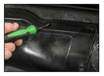
**9.** Using a T15 Torx Driver, remove the 19 screws that attach the Factory Trunk Panel to the vehicle.
