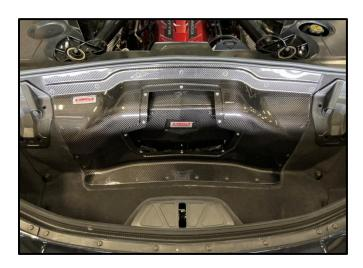
**24.** After all 19 screws are started, begin at the Top Center Screw and tighten the 19 screws using a T15 Torx Driver and **ONLY BY HAND**.
