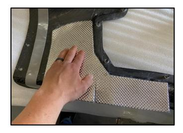
21. Realign the Heat Shield with the Trunk Panel recess. Do not allow the Heat Shield to touch the Carbon panel until it is properly aligned. The adhesive is aggressive and permanent. Gently press all over the upper portion of the heat shield to firmly attach it to the Carbon Panel.
