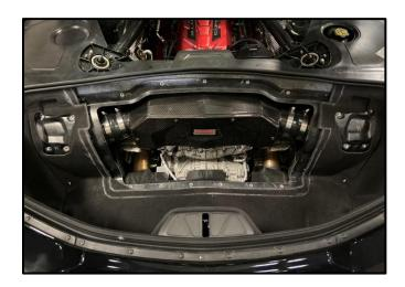
14. Place the Trunk Carpet back into the trunk and align it as if it were installed. Next, loosely install the Roof Storage Latches to ensure the carpet is properly positioned. Then gently set the CORSA Carbon Fiber Trunk Panel into position by aligning the screw holes with the threaded inserts.
