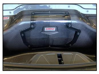
25. Using a 4mm Hex Wrench, remove the 10 preinstalled Window Screws and Rubber Washers. Next, place the window into the recess and reinstall the Window Screws and Rubber Washers. Start with the upper center screw then lower center screw. This will help align the window to the recess. Do not over tighten the screws. Only tighten BY HAND. The washers will provide constant pressure to keep the window in place and the gasket sealed to the carbon panel.
