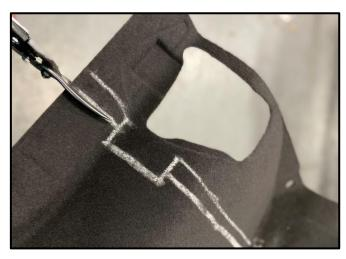
12. Using an Utility or Upholstery Knife, an Upholstery or Utility Shears, or combination of both, carefully cut the Trunk Carpet on the inside line made in Step 5. Follow the inner lines shown in the upper right image, by the Factory Roof Storage Latches. More carpet material is needed in these areas.
