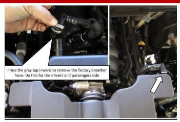
**1.** Press the gray tap inward to remove the factory driver breather hose. Repeat for passenger side.
