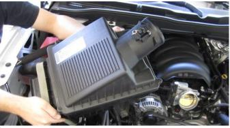
Remove the factory air box by pulling up and out.
