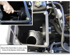
Mount the CORSA box in place using two of the factory 10mm bolts.
