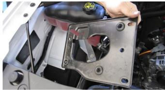
Remove the four 10mm bolts holding the air box **9**. mounting plate in place then remove the plate.
