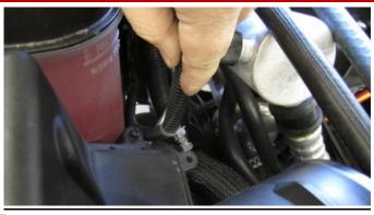
Remove the tree rivet holding the MAF harness to the air box.
