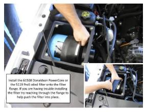
**3.** Install air filter, onto the filter flange. If you are having trouble installing the filter try reaching through the flange to help push the filter into place.
