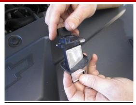
13. Install the supplied CORSA MAF gasket.
