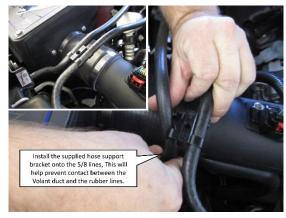
17. Install the supplied hose support bracket onto the 5/8 lines. This will help prevent contact between the CORSA duct and the rubber lines.
