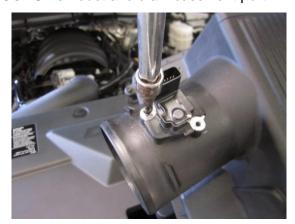
**11.** Remove the torx bits holding the MAF into place using the supplied bit.
