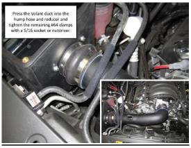
**8.** Press the CORSA duct into the hump hose and reducer and tighten the remaining #64 clamps with a 5/16 socket or nut driver.
