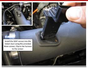
14. Install the MAF sensor into the CORSA duct using the provided 4mm screws. Clip in the harness to the sensor.
