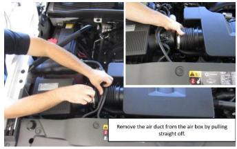
Remove the air duct from the air box by pulling straight off.
