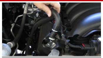
Remove the factory driver and passenger side breather hose from the engine.
