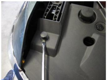
**10.** Remove the four tabs holding the shroud onto the passenger side using a flathead screw driver or pry tool.
