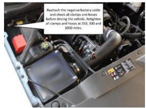
**18.** Reattach the negative battery cable and check all clamps and hoses before driving the vehicle. Retighten all clamps and hoses at 150, 300, and 1,000 miles.
