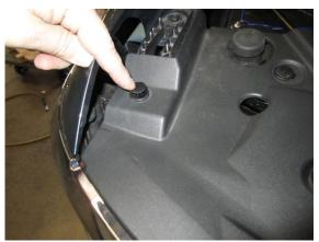
**16.** Reinstall the shroud support pins.
