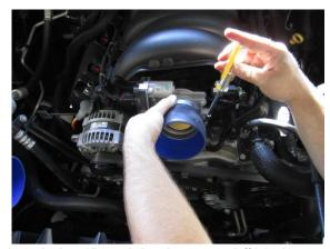
**6.** Attach the 4" straight sleeve and #64 clamp using a 5/16 socket or nut driver.
